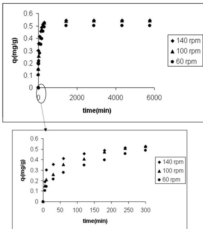
**Fig. 4.** Effect of agitation speed on the sorption of Cr(VI) by *E. coli* loaded clinoptilolite rich mineral (concentration: 10 mg/L, temperature: 25 °C, particle size: 25–106  $\mu\text{m}$ ).
