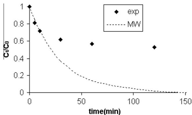
Fig. 6. Comparison of theoretical and experimental concentration decay curve for the *E. coli* loaded clinoptilolite rich mineral (concentration: 10 mg/L, agitation speed: 140 rpm, particle size: 25–106  $\mu\text{m}$ , temperature: 25  $^{\circ}\text{C}$ ).
