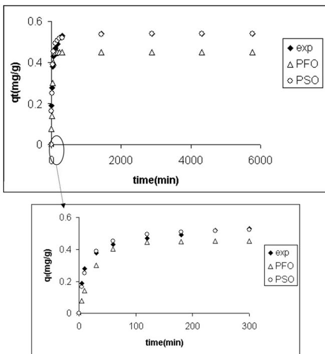
Fig. 8. Comparison of the experimental and reaction model results for *E.Coli* loaded clinoptilolite rich mineral (concentration: 10 mg/L, agitation speed: 140 rpm, particle size: 25–106  $\mu\text{m}$ , temperature: 25  $^{\circ}\text{C}$ ).
