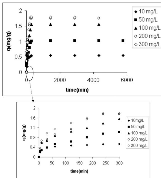
Fig. 3. Effect of initial concentration on the sorption of Cr(VI) by *E. coli* loaded clinoptilolite rich mineral (temperature: 25 °C, agitation speed: 140 rpm, particle size: 25–106 μm).
