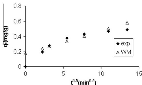
Fig. 7. Comparison of theoretical and experimental Weber–Morris model results for the *E. coli* loaded clinoptilolite rich mineral (concentration: 10 mg/L, agitation speed: 140 rpm, particle size: 25–106  $\mu\text{m}$ , temperature: 25  $^{\circ}\text{C}$ ).
