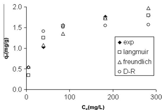
**Fig. 11.** Equilibrium isotherm for Cr(VI) sorption by *E. coli* loaded clinoptilolite rich mineral at 25 °C.
