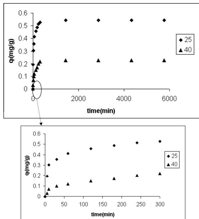
**Fig. 5.** Effect of temperature on the sorption of Cr(VI) by *E. coli* loaded clinoptilolite rich mineral (concentration: 10 mg/L, agitation speed: 140 rpm, particle size: 25–106  $\mu\text{m}$ ).
