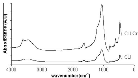
Fig. 10. FTIR results of parent mineral and after Cr(VI) sorption.
