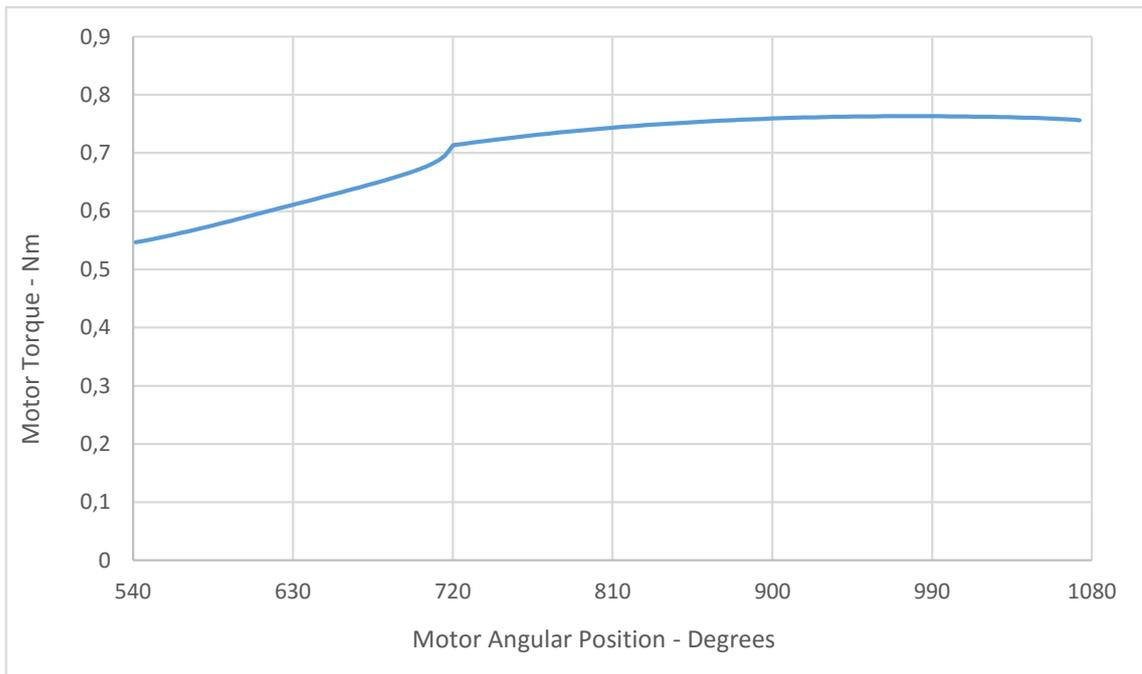
Figure 39. Motor Torque for Cable Actuation in Oblique Plane
