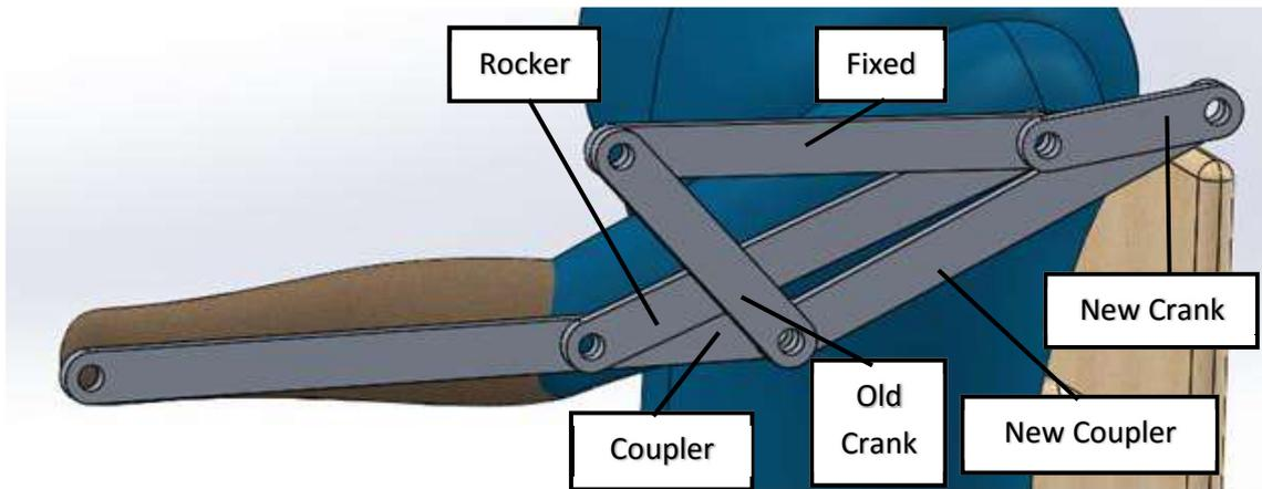
Figure 21. Mechanism with Extra Dyad in Vertical Plane
