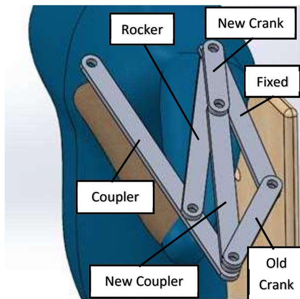
Figure 22. Mechanism with Extra Dyad in Oblique Plane
