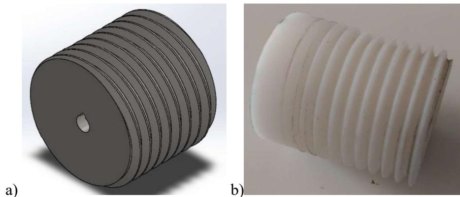
Figure 46. Motor Pulley: a) the CAD Model and b) the Manufactured Model
