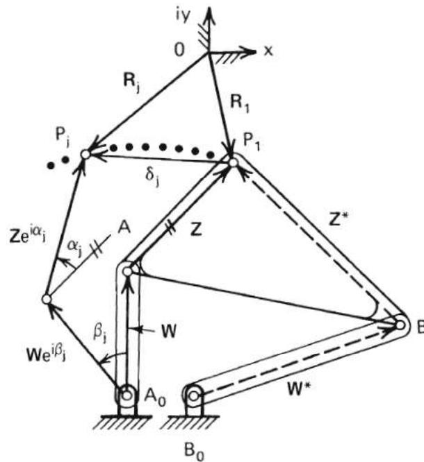
Figure 14. Motion Generation Synthesis of the Four-Bar Linkage [34]
