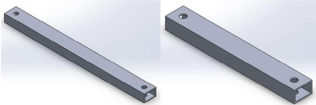
Figure 44. Rocker Link (Left) and Crank Link (Right)
