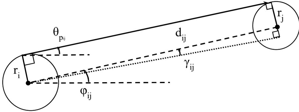
Figure 30. Parameters of Cable Angle Calculations for Multi-Pulley Solution
