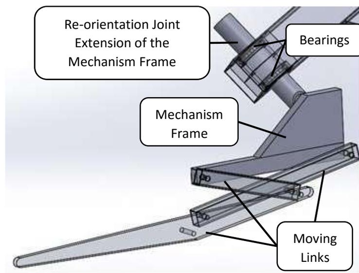
Figure 42. The Mechanism Frame Design before Cable Actuation
