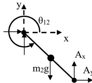
Figure 33. FBD of the Crank Link
