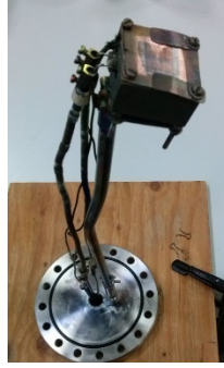
Figure 3. 6. Heating holder of the RF magnetron sputtering system.
