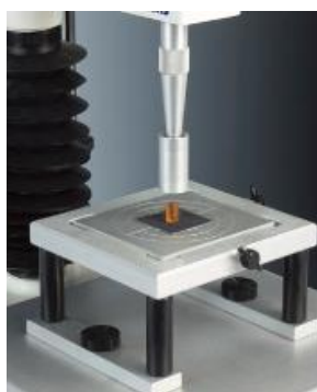
Figure 3.1. Compression test set up (Source: http://www.stablemicrosystems.com )
