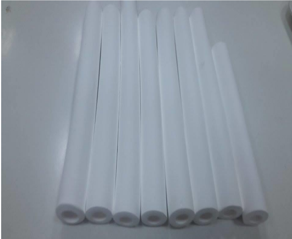
Figure 5.7. Tubular alumina ceramic membrane supports.
