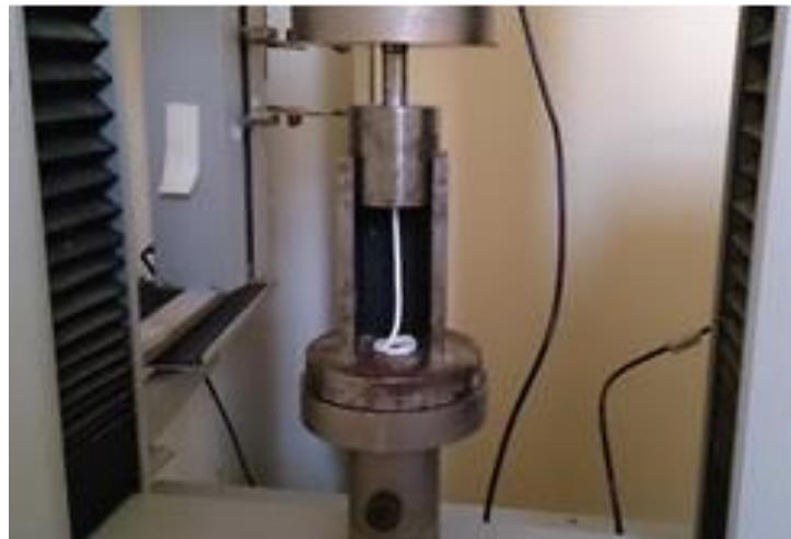
Figure 5.1. Extrusion of ceramic pastes in the mechanical test device (Testometric SN 500-526 ) with orifice die.
