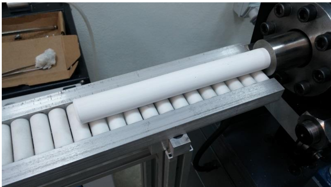
Figure 5.6. Extrusion of tubes from the piston extruder.
