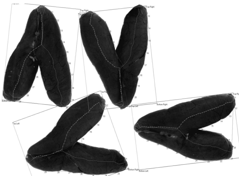
Figure 9. Example of medial axis determination of the two sides of the roe by using the “distance transform” method. Depending on the side, placement, and orientation, the length of the same side varied.
