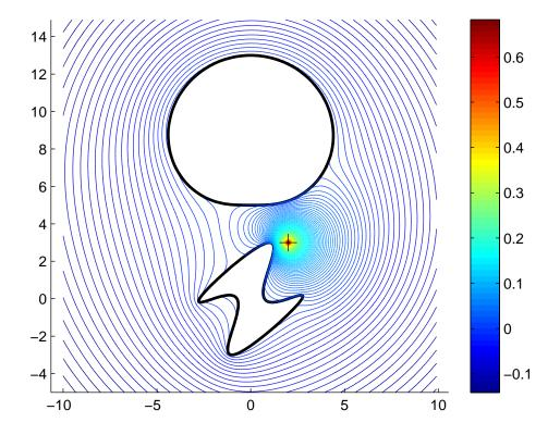
Figure 6.4. Equipotential lines of total field for a monopole
