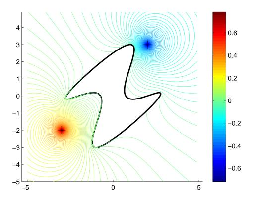
Figure 6.3. Equipotential lines of total field for a dipole for one domain
