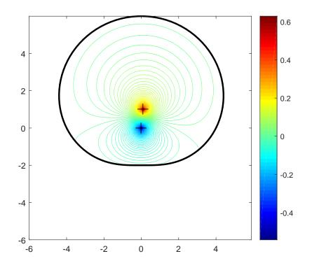
Figure 6.9. Equipotential lines of total field for a dipole
