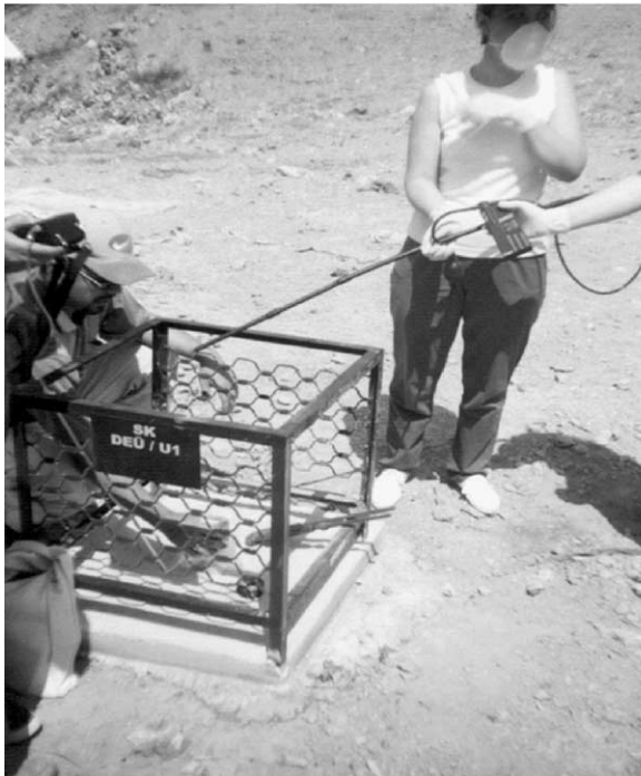
Fig. 2. Photograph and schematic of completed well No. SK-U1 for gas measurement (Onargan and Kucuk, 2000).
