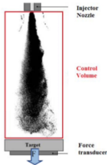
Figure 2.9. Scheme of control volume for momentum flux analysis. Source: (Postrioti et al., 2011)
