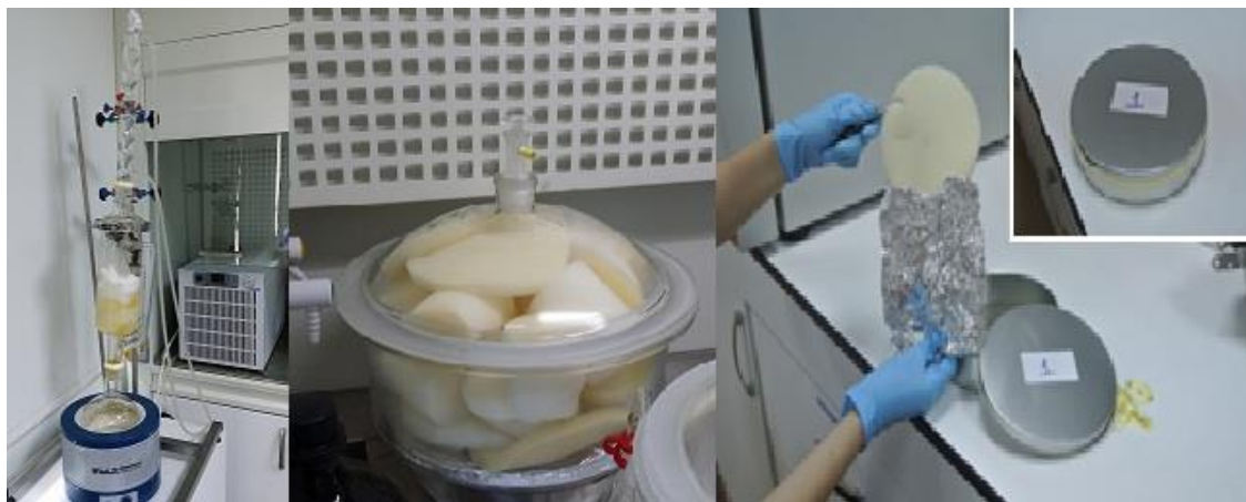
Figure 3.2. Cleaning and storage procedures of PUF discs
