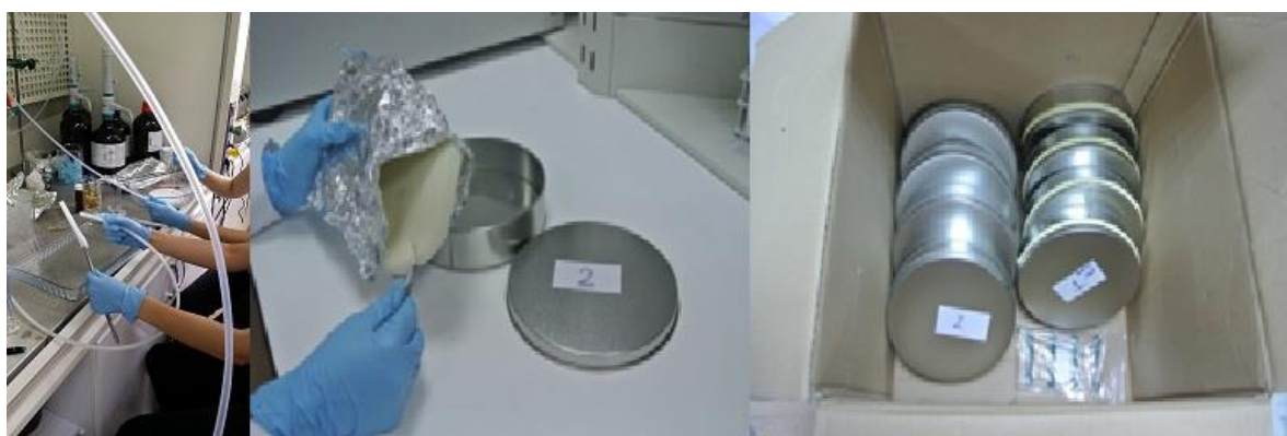
Figure 3.4. Injection of deuration chemicals on to PUFs and storage of boxes
