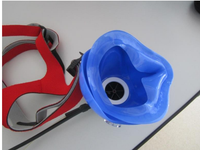
Figure 5.6. Facemask and flowmeter of gas analyser
