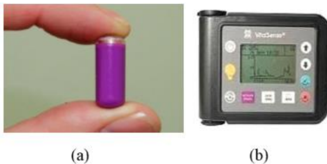
Figure 5.8. The ingestible thermal sensor(a) and data logger(b) of core body temperatures measurement device
