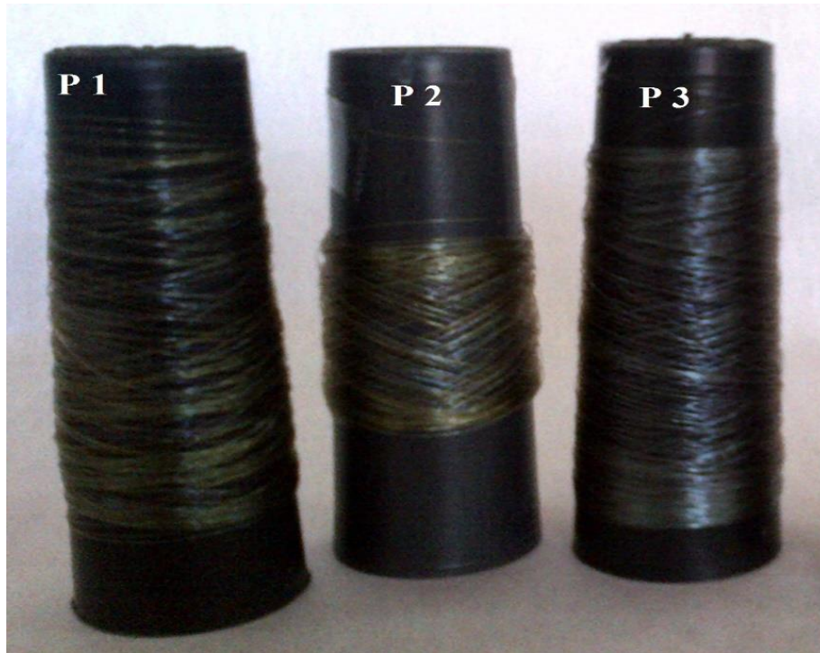
Figure 4.2. Pilot scale test works on ITO deposition on PA fibers
