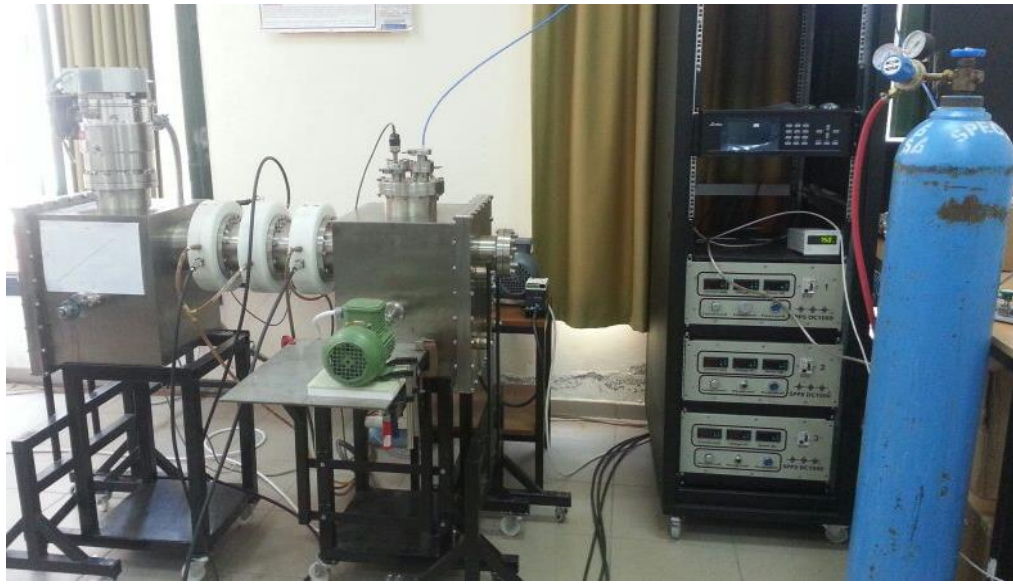
Figure 3.9. Roll to roll inverted cylindrical magnetron sputtering system which is used in the scope of the thesis.
