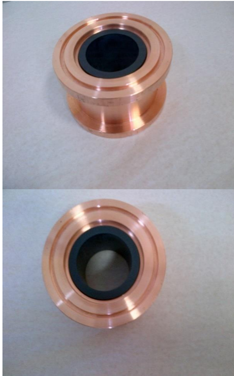
Figure 3.5. Special designed cylindrical ITO target.
