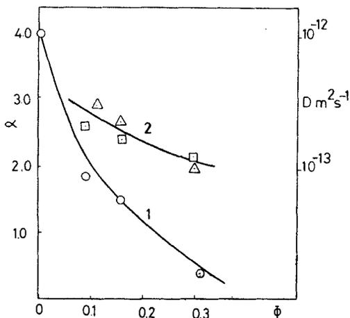
FIG. 2 Curve 1: The ratio of the equilibrium amount of dye remaining in solution to the amount of dye adsorbed on the pellets,  $\alpha$ , versus zeolite volume fraction of the composites ( $\odot$ ). Curve 2: Effective diffusion coefficient of methylene blue in composite versus volume fraction of zeolite, calculated from the solution ( $\Delta$ ) and calculated from the diffusion front in the solid ( $\square$ ).
