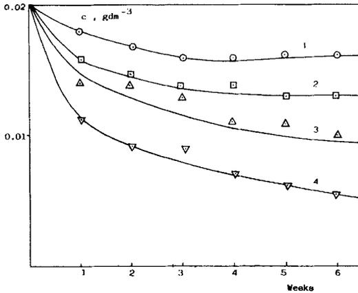
FIG. 5 Methylene blue concentration versus time for adsorption rate experiments for composites having (1, ○) 0.0, (2, □) 0.1, (3, △) 0.16, and (4, ▽) 0.30 volume fractions of zeolite.
