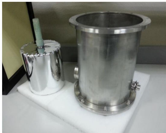
Figure 3.19. Liquid nitrogen chamber surrounding with metalize film
