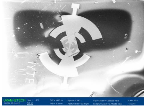
Figure 4.8. SEM image of log-periodic antenna by e-beam lithography on Bi2212 single crystal
