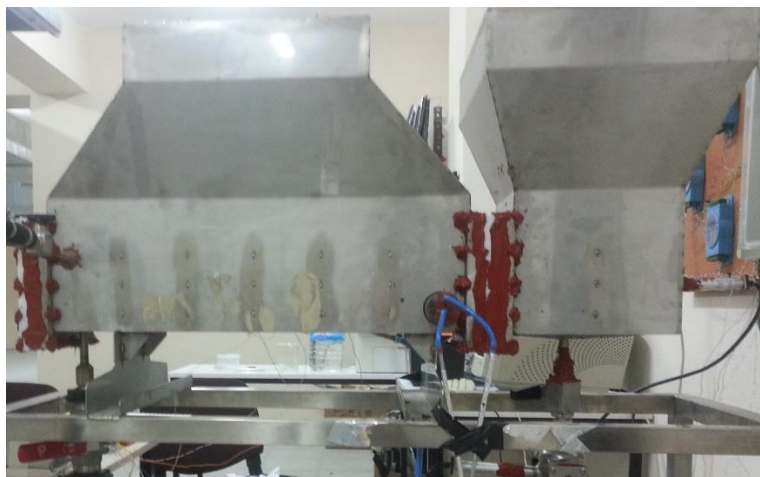
Figure 5.16. The view of the evaporator is located near the adsorbent bed after the revision of experimental setup.
