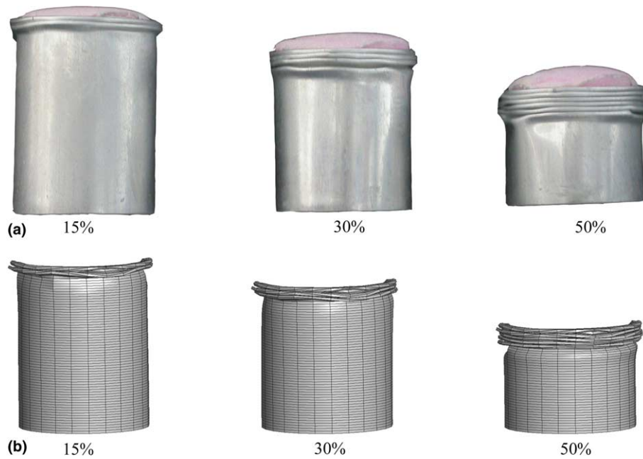
Fig. 11. Deformation histories of 25-mm foam-filled ( 27.8 \text{ kg m}^{-3} ) tube at various percent deformation ratios: (a) experimental and (b) numerical.
