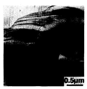
Figure 5. Crack propagation from porosity in SiC particle.
