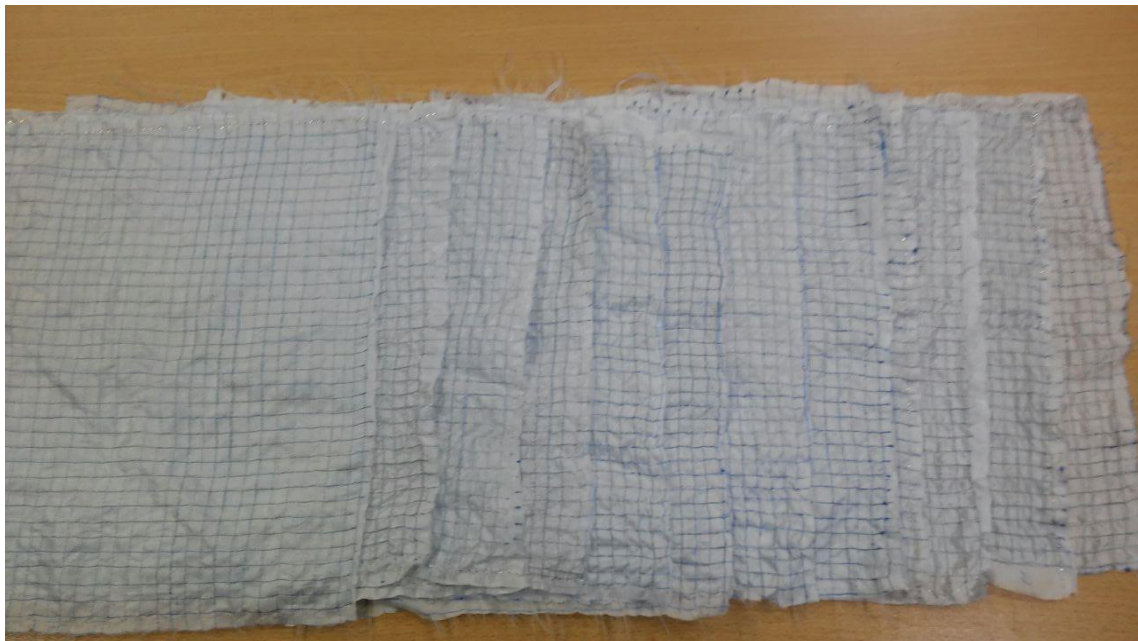
Figure 4.7. 35 x 35 cm fabrics woven with 10 mm interval horizontal and vertical
