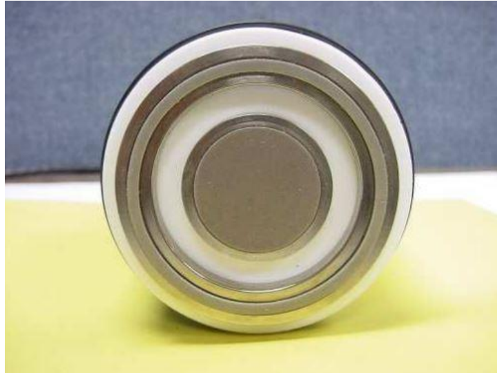
Figure 4.6. Surface resistance measurement test probe
