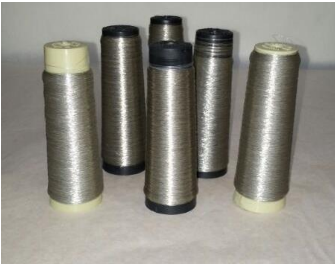
Figure 5.2. Silver thin film coated fibers winded on rolls
