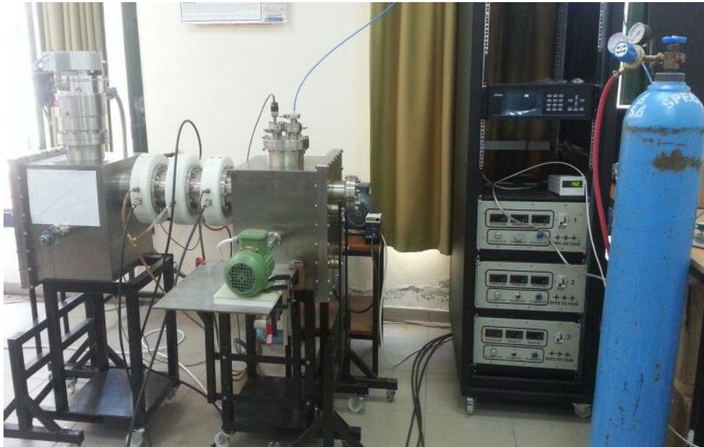
Figure 4.1. Our inverted cylindrical magnetron sputtering system
