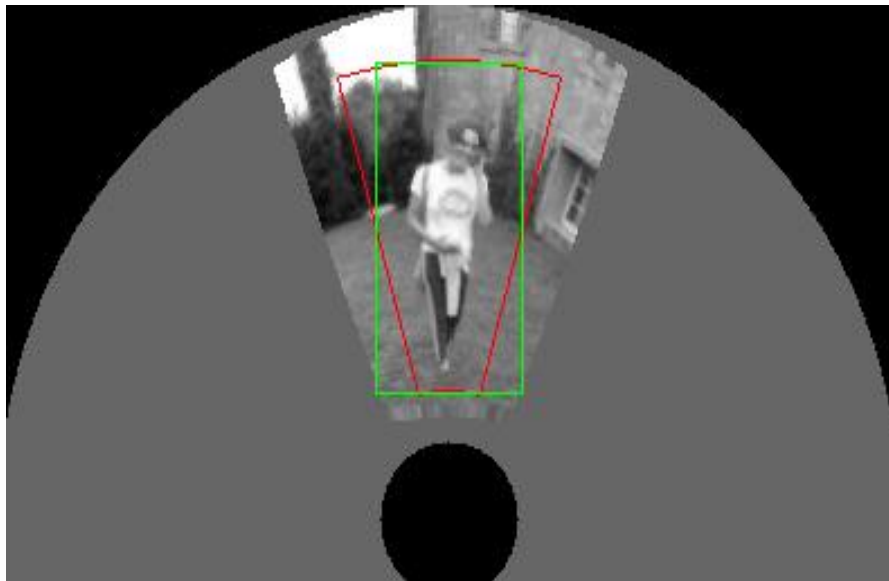
Figure 5.3. Depiction of the regular HOG window (green rectangle) and the proposed window (red doughnut slice) on an omnidirectional image artificially created by projecting a perspective image from INRIA person dataset.
