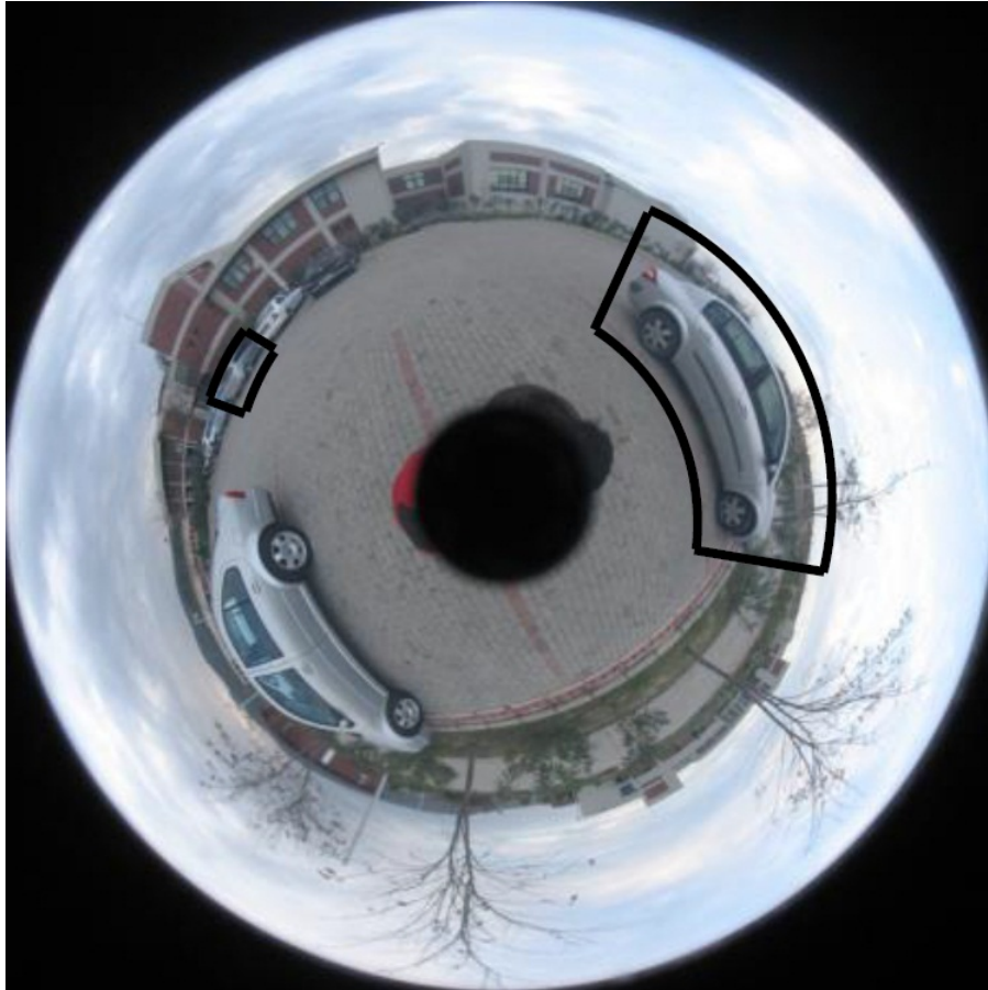
Figure 4.4. Two cars in the omnidirectional image are indicated with black frames. The one close to the camera covers a larger area and it should be searched with a more bent sliding window, the other one is far away and it should be search with a more straight sliding window
