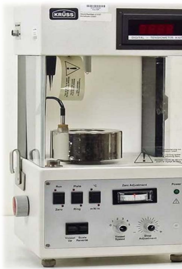
Figure 3.3. A Krüss model digital tensiometer (K10ST) used for surface tension measurements.
