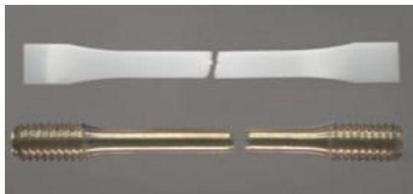
Figure 4.1. Tensile test specimens having (a) rectangular and (b) round cross section [45]
