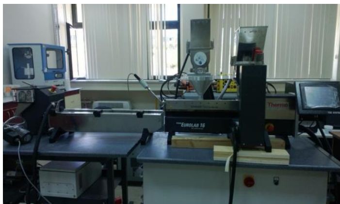
Figure 5.5. Thermofisher (Eurolab 16 mm) twin-screw extruder
