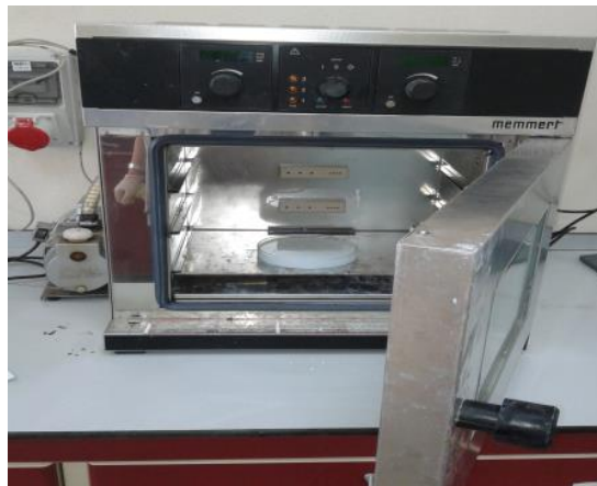
Figure 5.4. Air-circulating oven used in drying process
