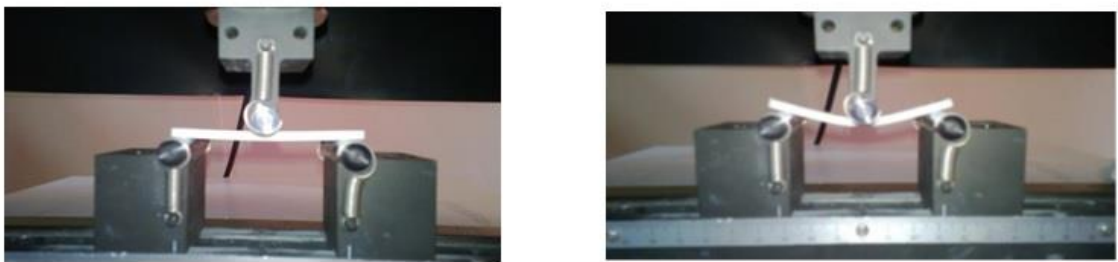
Figure 5.2. Specimen under three point bending, (a) before loading, (b) during loading
