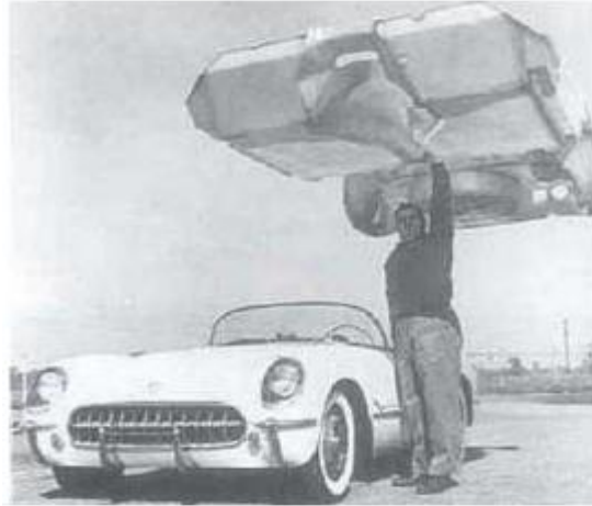
Figure 2.8. 1953 Chevrolet Corvette- the first production car to use structural composite materials.
