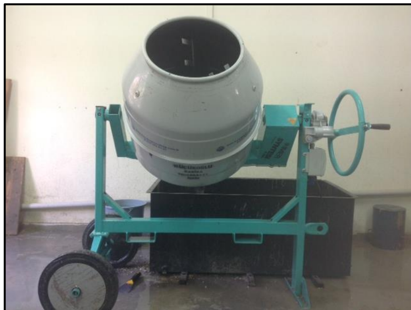
Figure 4.9. Rotating drum mixer with 100 Liter capacity
