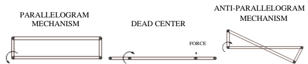
Fig. 04 Assembly mode change through the dead center
