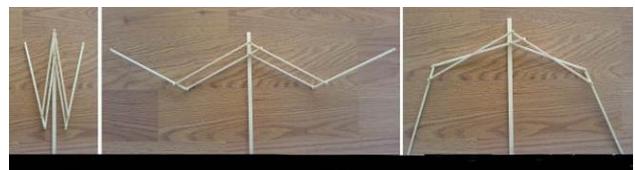
Fig. 05 Planar linkage unit in compact, open and closed form.
