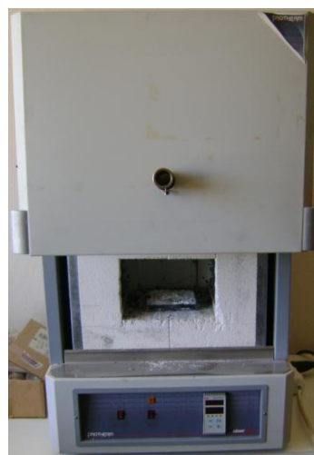
Figure 5.2. The picture of furnace used in the heat treatment process of tension test specimens.
