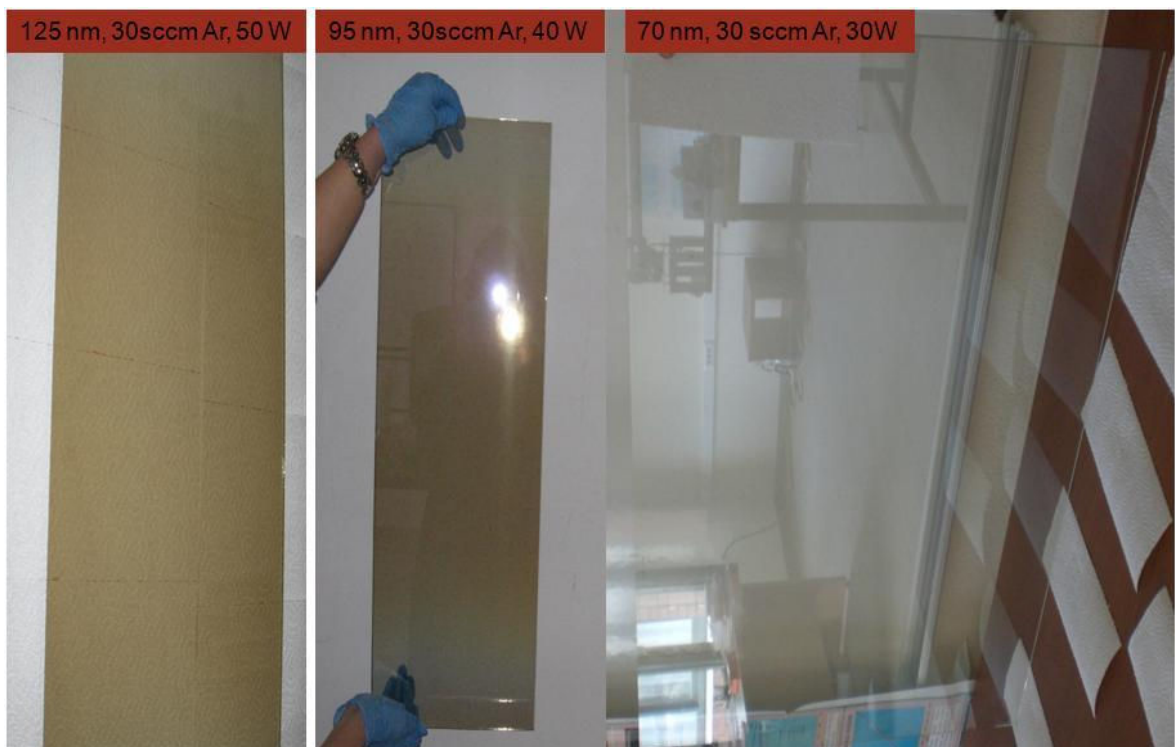
Figure 3.4. ITO coated large area glass
