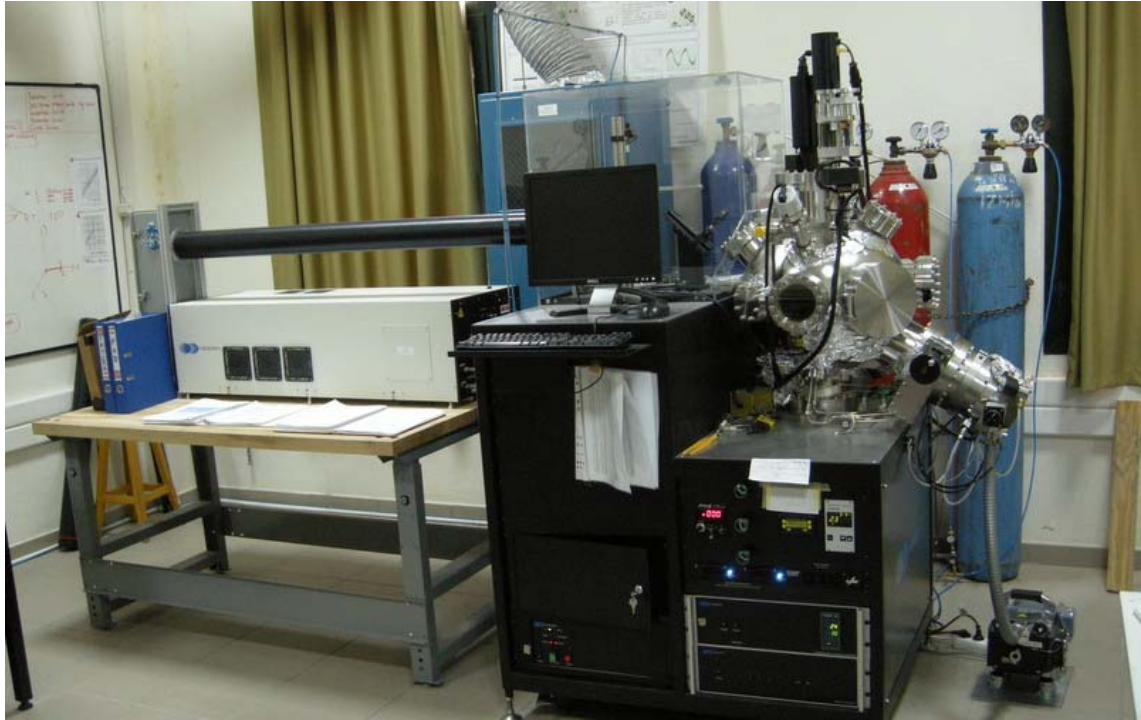
Figure 4.3. The schematics of the PLD set up used for this work
