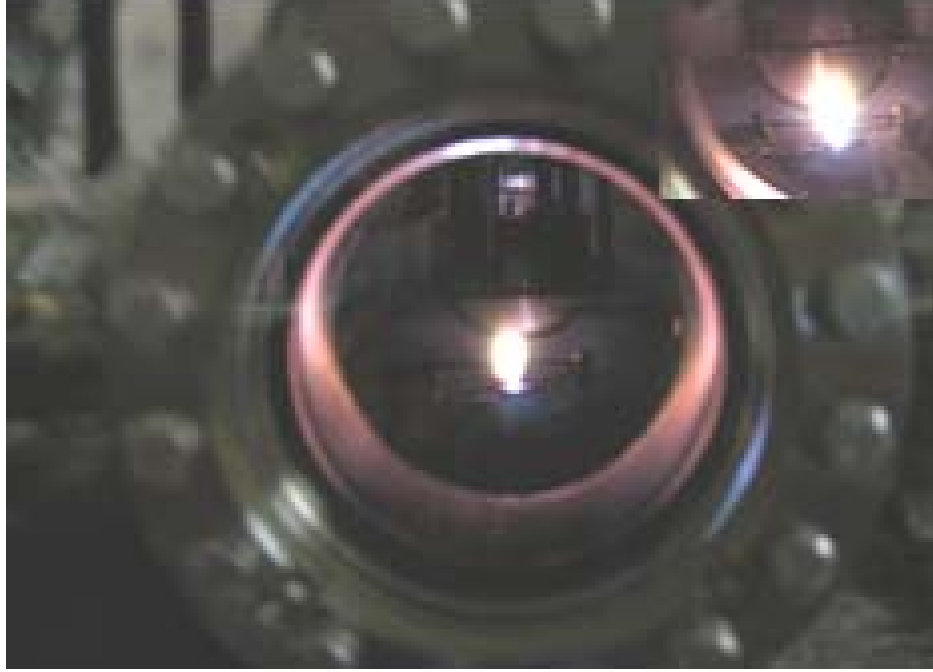
Figure 4.6. Plume ejected from YBCO during deposition process
