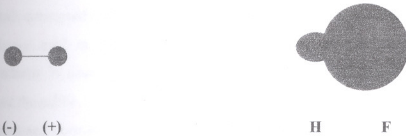
Fig. 1.10 Electrical Dipole effect in HF molecule
