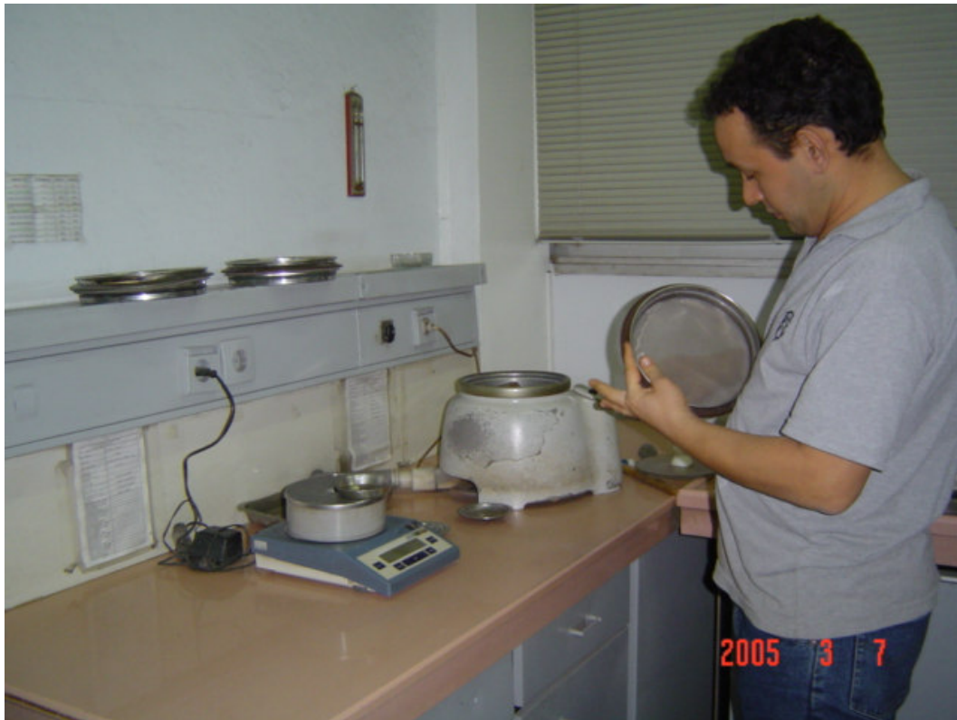
Figure B.2. Sieve equipment used in the local plant.
