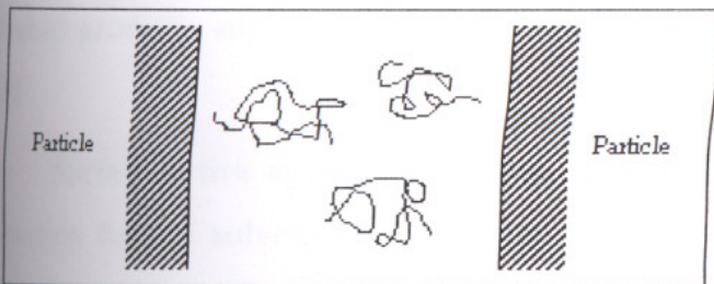
(a) Depletion stabilization at separation greater than the diameter of the polymer coil.
