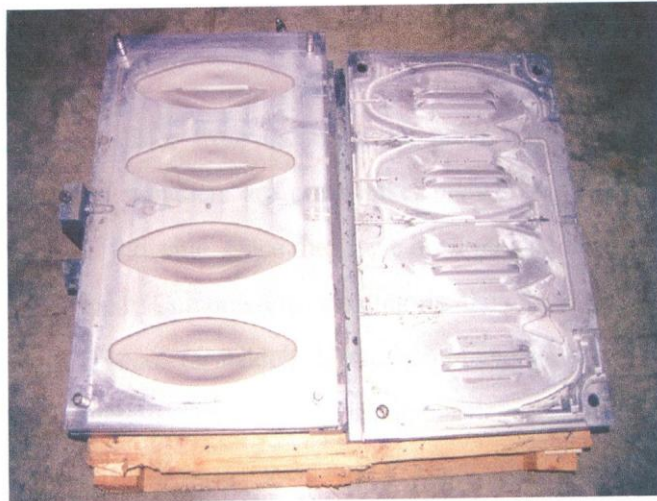
Figure 2.12: Soft expanded polyurethane resin is formed in injection molds. (Byars M.,1998, p:52 )
