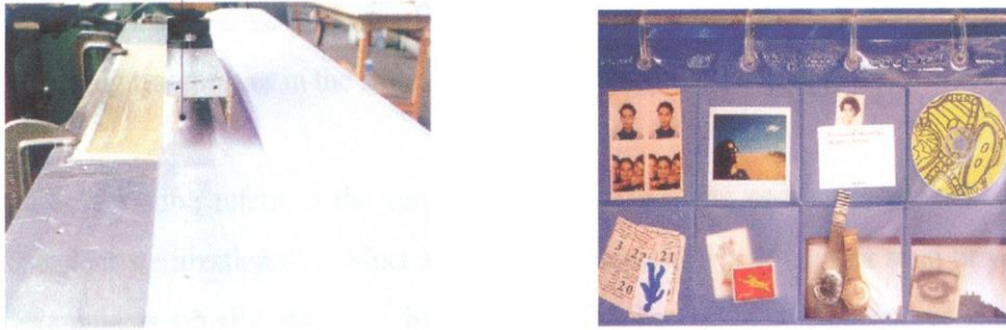
Figure 2.7: Left, the doubled-over top edges is high frequency heat sealed. Right, close view of object PVC- polyvinylchloride . (Byars M., 1998, p:26 )
