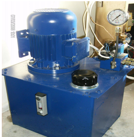
Figure 4.5. Hydraulic Power Unit
