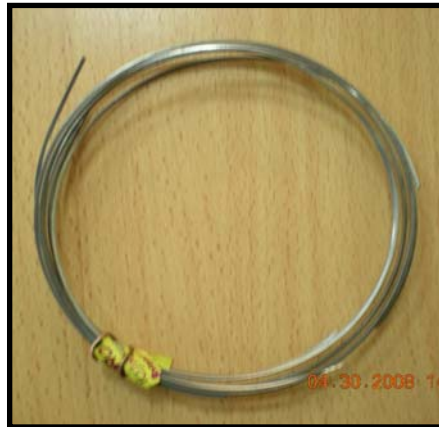
Figure 4.19. \text{MgB}_2/\text{Fe} Wire Produced by in situ PIT Method
