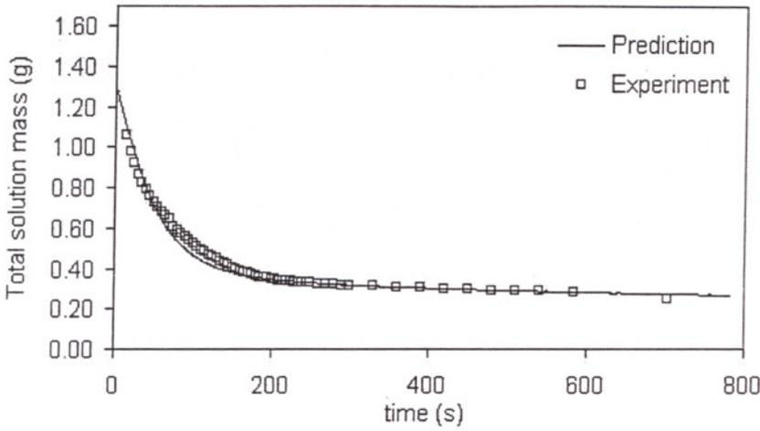
Figure 6.1. Predicted(-) and measured ( ) total solution mass as a function of time for a membrane cast from a CA/Acetone/Water solution for case R1.
