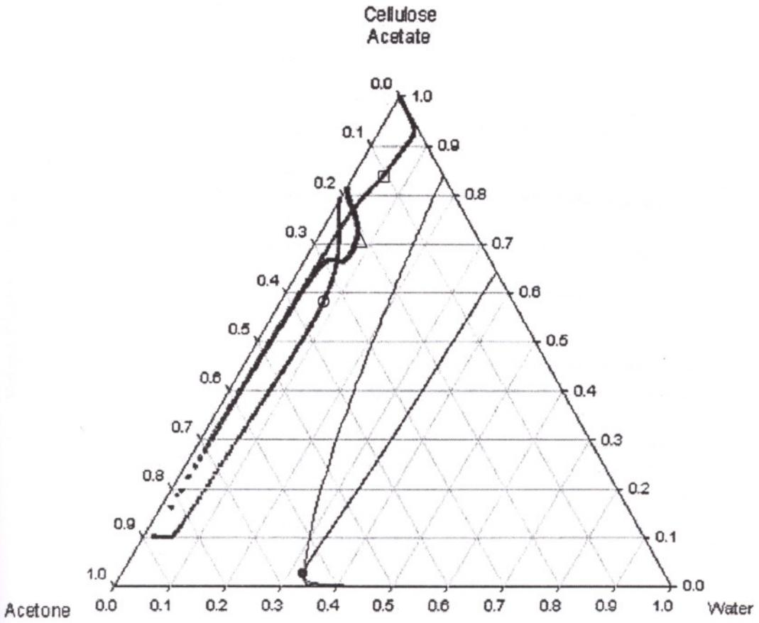
Figure 6.18. Concentration paths of water, acetone and CA for case R6 (O: solution/substrate interface, □: solution/air interface, Δ: point just below solution/air interface).
