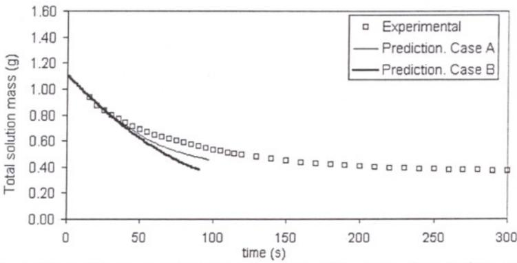
Figure 6.32. Experimental corresponding to case R2, and simulation results for total solution mass as a function of time. The line corresponds to full model, whereas the dashed solid line represents the solution when the cross diffusion coefficients are assumed to be negligible.
