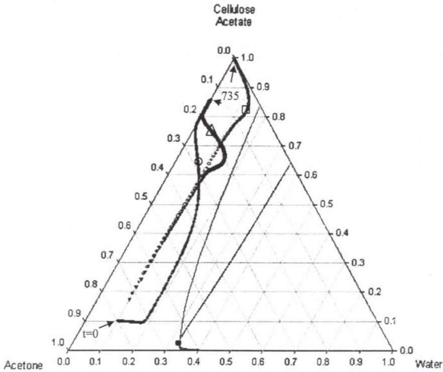
Figure 6.29. Concentration paths of water, acetone and CA for case R10 (O: solution/substrate interface, □: solution/air interface, Δ: point just below solution/air interface).
