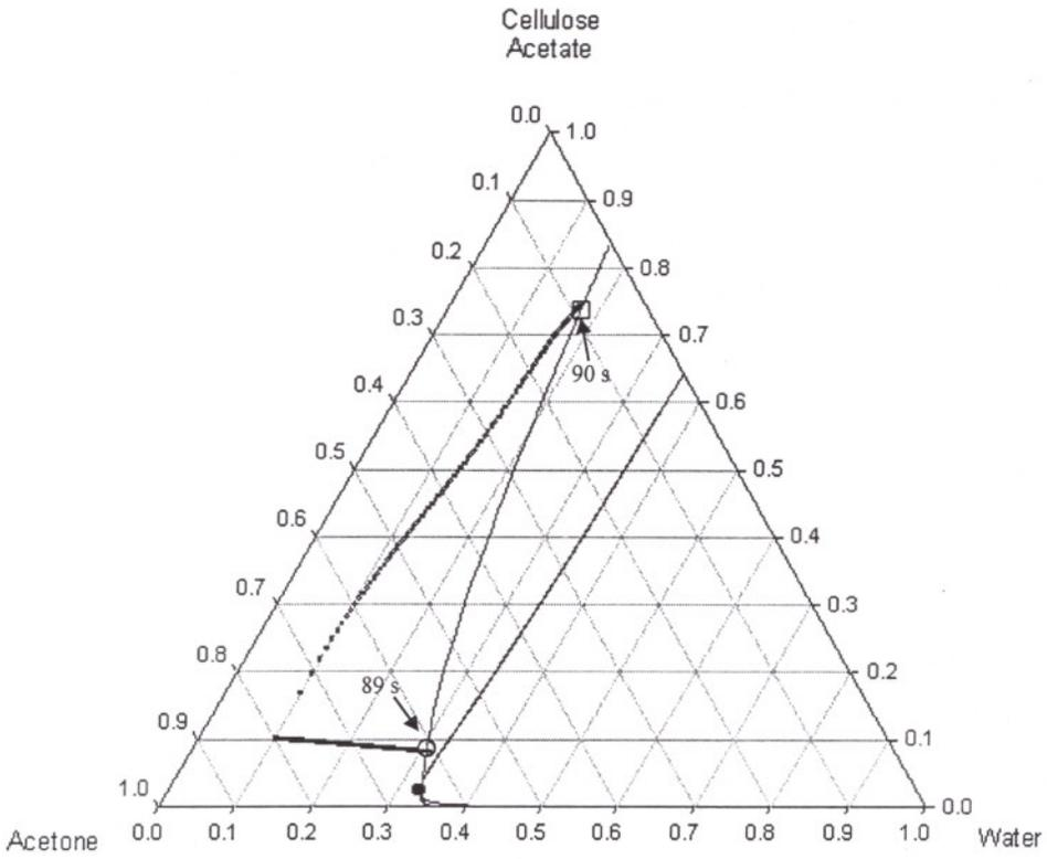
Figure 6.34. Concentration paths of water, acetone and CA for case A (○: solution/substrate interface, □: solution/air interface).
