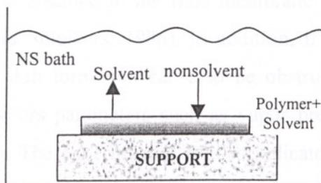
Figure 3.5. Schematic representation of the immersion step.
