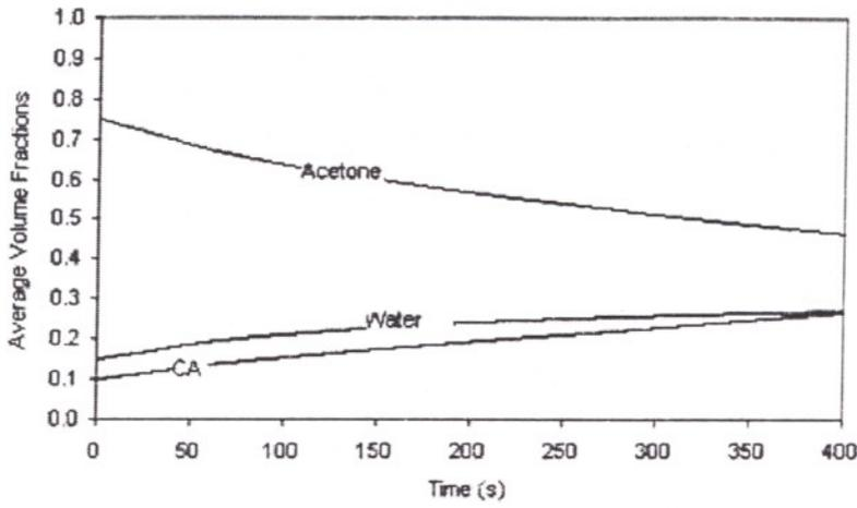
Figure 6.15. Average volume fractions of water, acetone and CA during membrane formation for case R5.
