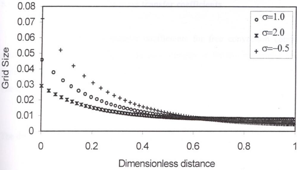
Figure 5.3. Variation of grid sizes with  $\sigma$  ( $\epsilon = -4.0$  and # Grid Points=100)
