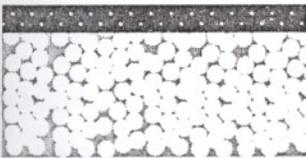
porous layer and dense layer of a different material: composite
