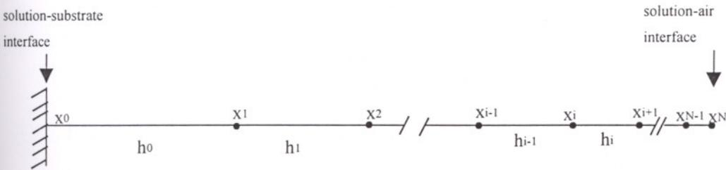
Figure 5.2. Illustration of variable grid spacing for N grid points.
