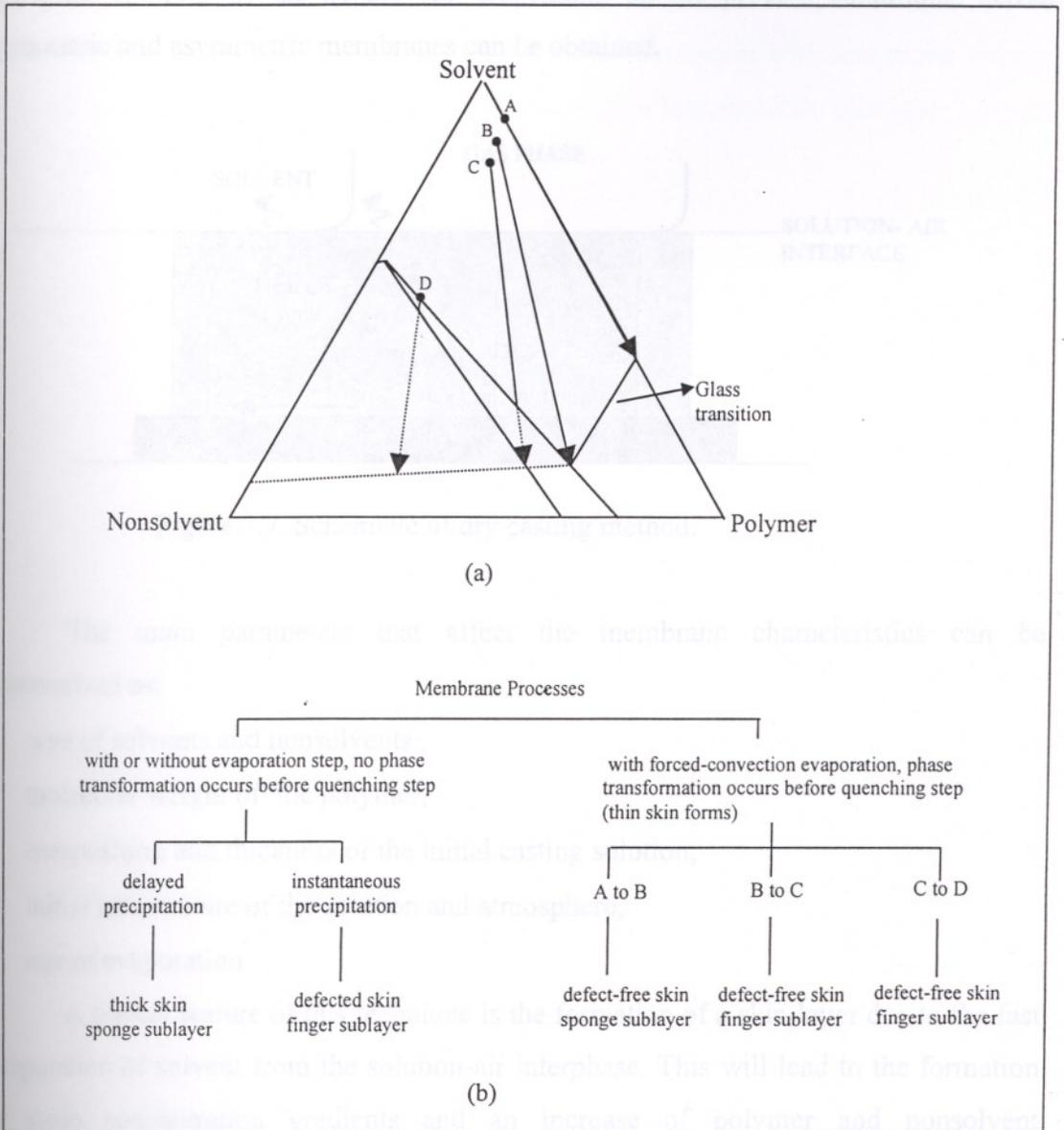
Figure 3.6. (a) Ternary phase diagram and concentration paths during membrane formation, (b) morphology-process relationship. (Reproduced from Tsay and McHugh, 1992)
