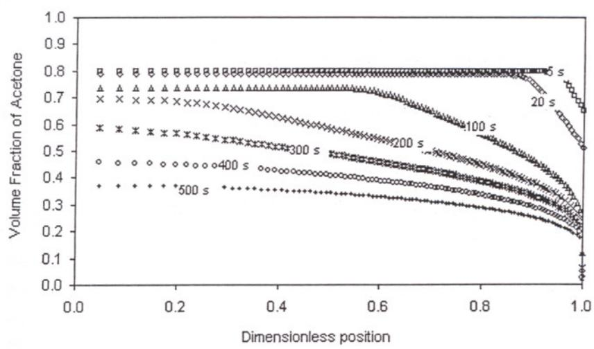
Figure 6.7. Volume fraction profiles of acetone for case R4.
