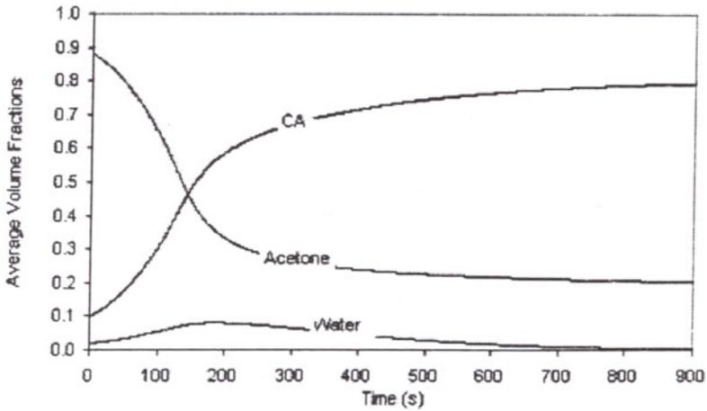
Figure 6.22. Average volume fractions of water, acetone and CA during membrane formation for case R6.
