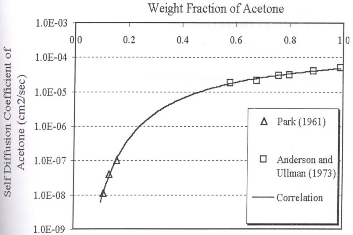
Figure 4.2. The self diffusion coefficient of acetone in cellulose acetate as a function of weight fraction. Comparison of the experimental data (Anderson and Ullman 1973, Park 1961) with the calculated self diffusion coefficients.
