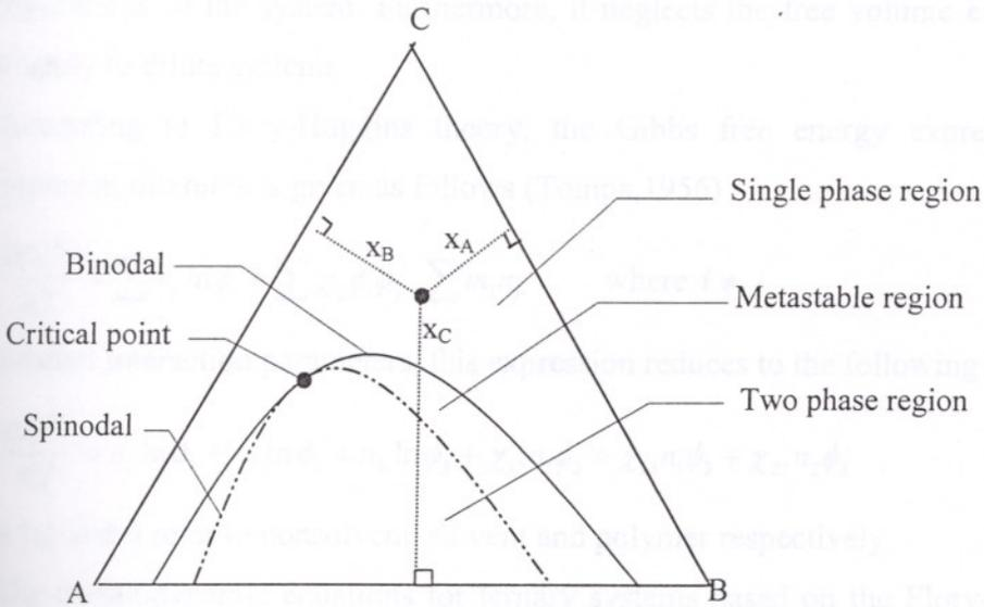
Figure 3.4. Sketch of change of Gibbs free energy surface for a ternary solution and ternary phase diagram.
