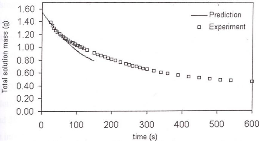
Figure 6.3. Predicted(-) and measured ( ) total solution mass as a function of time for a membrane cast from a CA/Acetone/Water solution for case R3.
