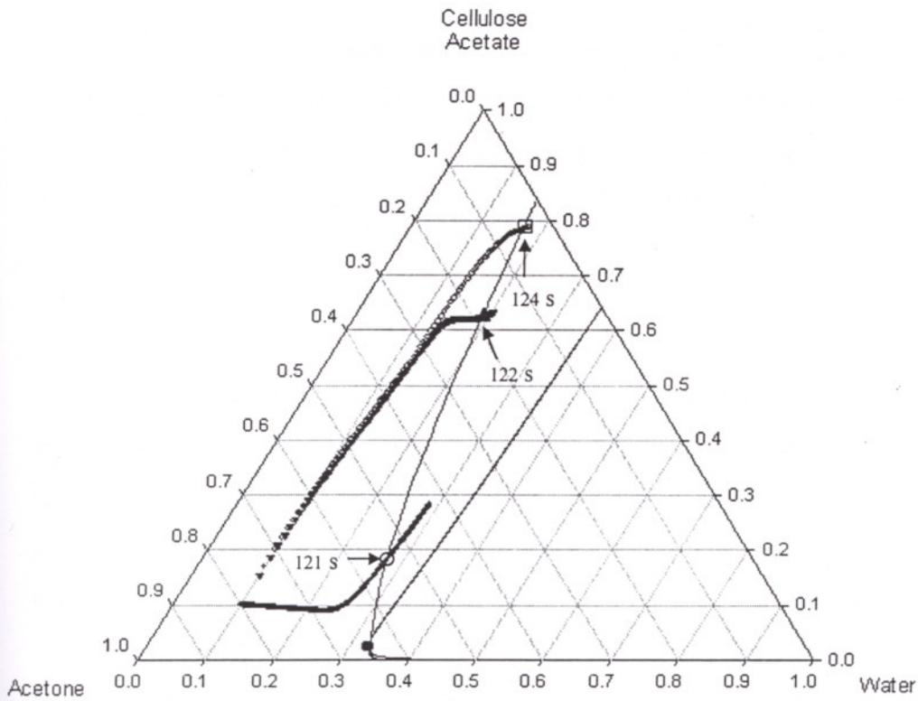
Figure 6.25. Concentration paths of water, acetone and CA for case R7 (O: solution/substrate interface, □: solution/air interface, Δ: point just below solution/air interface).
