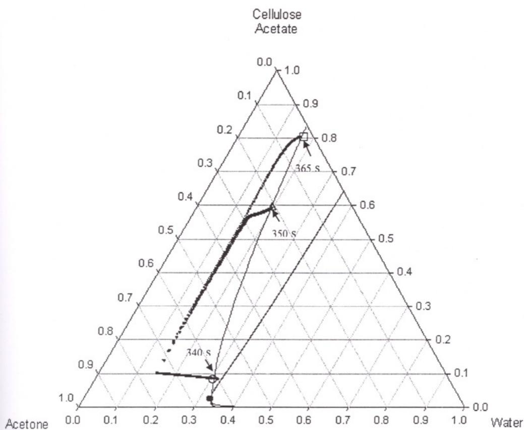
Figure 6.11. Concentration paths of water, acetone and CA for R5 (O: solution/substrate interface, □ solution/air interface, Δ: point just below solution/air interface).
