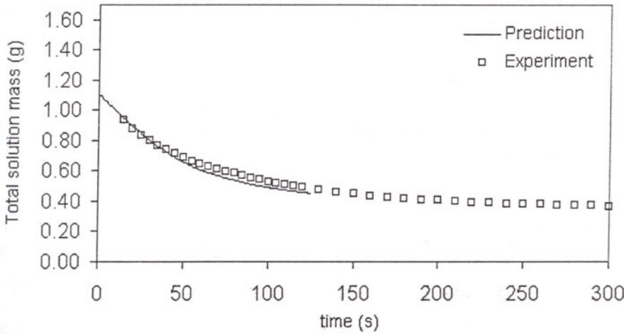
Figure 6.2. Predicted(-) and measured ( ) total solution mass as a function of time for a membrane cast from a CA/Acetone/Water solution for case R2.
