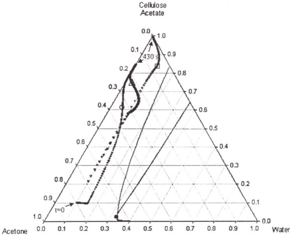
Figure 6.30. Concentration paths of water, acetone and CA for case R11 (O: solution/substrate interface, □: solution/air interface, Δ: point just below solution/air interface).
