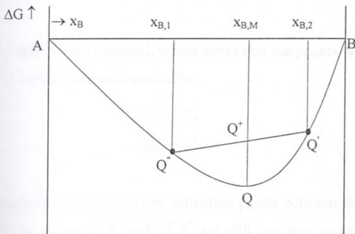
Figure 3.2. Free energy curve versus composition for a binary mixture.
