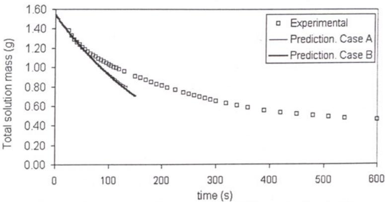
Figure 6.33. Experimental corresponding to case R3, and simulation results for total solution mass as a function of time. The line corresponds to full model, whereas the dashed solid line represents the solution when the cross diffusion coefficients are assumed to be negligible.
