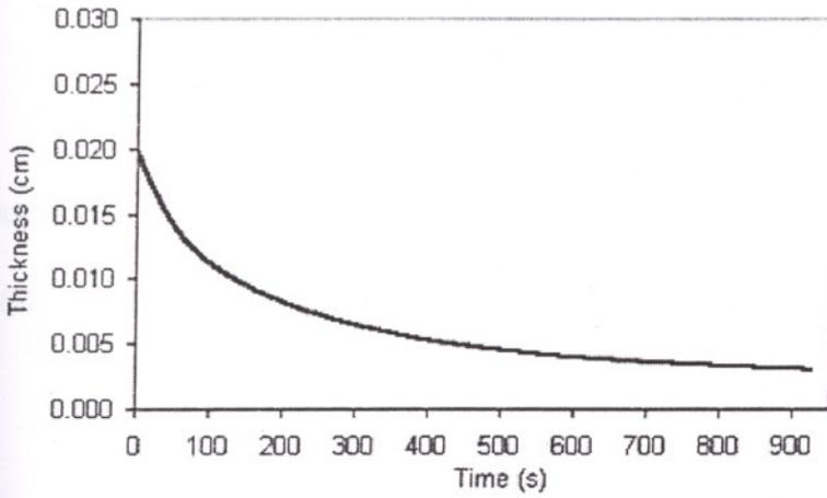
Figure 6.9. Thickness of the solution during membrane formation for case R4.
