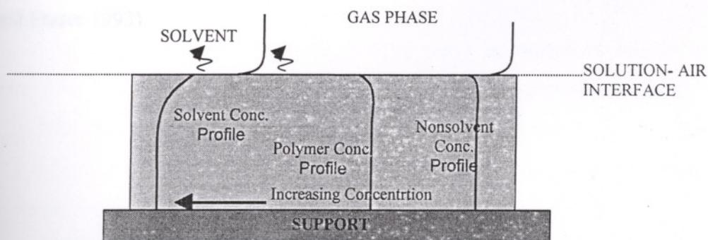
Figure 3.7. Schematic of dry casting method.
