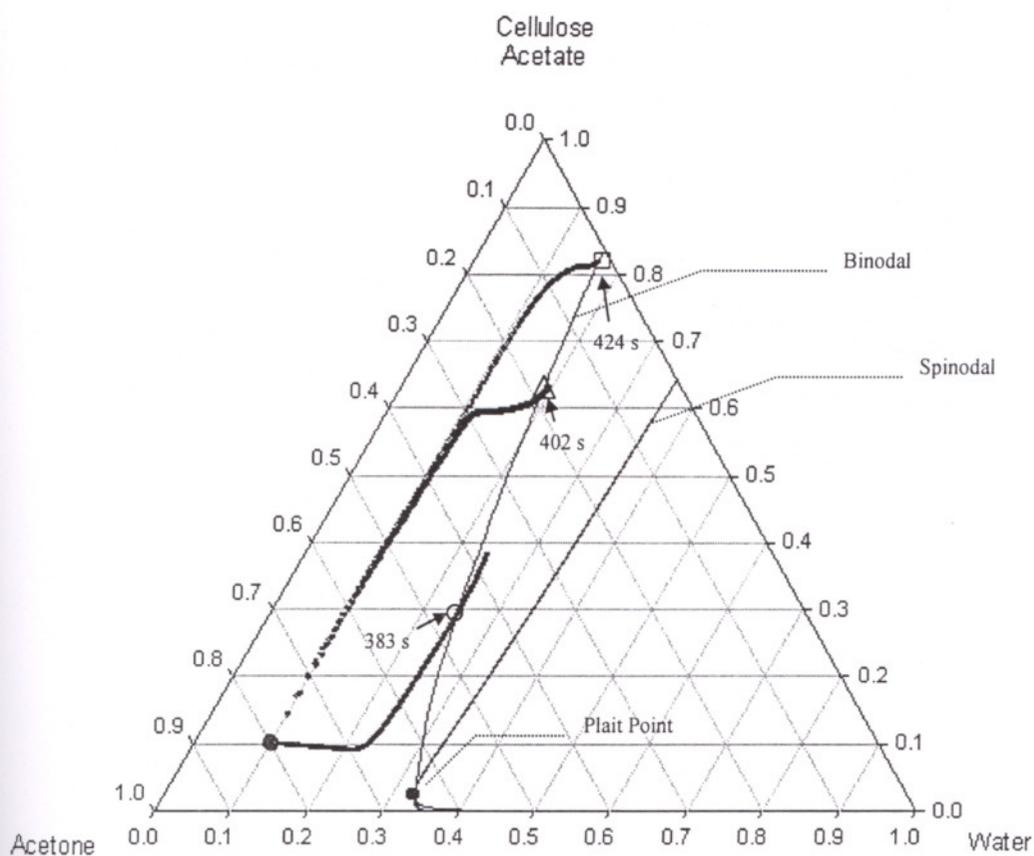
Figure 6.4. Concentration paths of water, acetone and CA for case R4 (O: solution/substrate interface,  $\square$ : solution/air interface  $\Delta$ : point just below solution/air interface).
