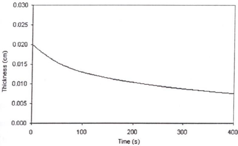
Figure 6.16. Thickness of the solution during membrane formation for case R5.
