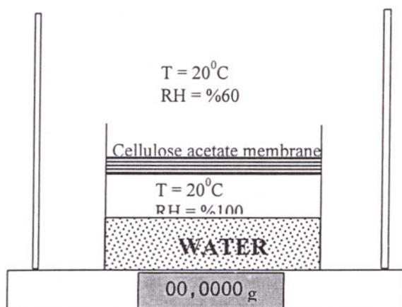
Figure 7.1. Schematic of experimental setup used in measuring water vapor permeability coefficients.
