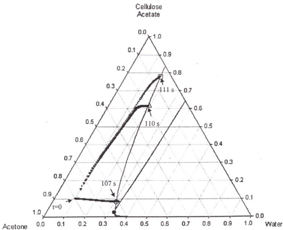
Figure 6.28. Concentration paths of water, acetone and CA for case R2 (O: solution/substrate interface, □: solution/air interface, Δ: point just below solution/air interface).
