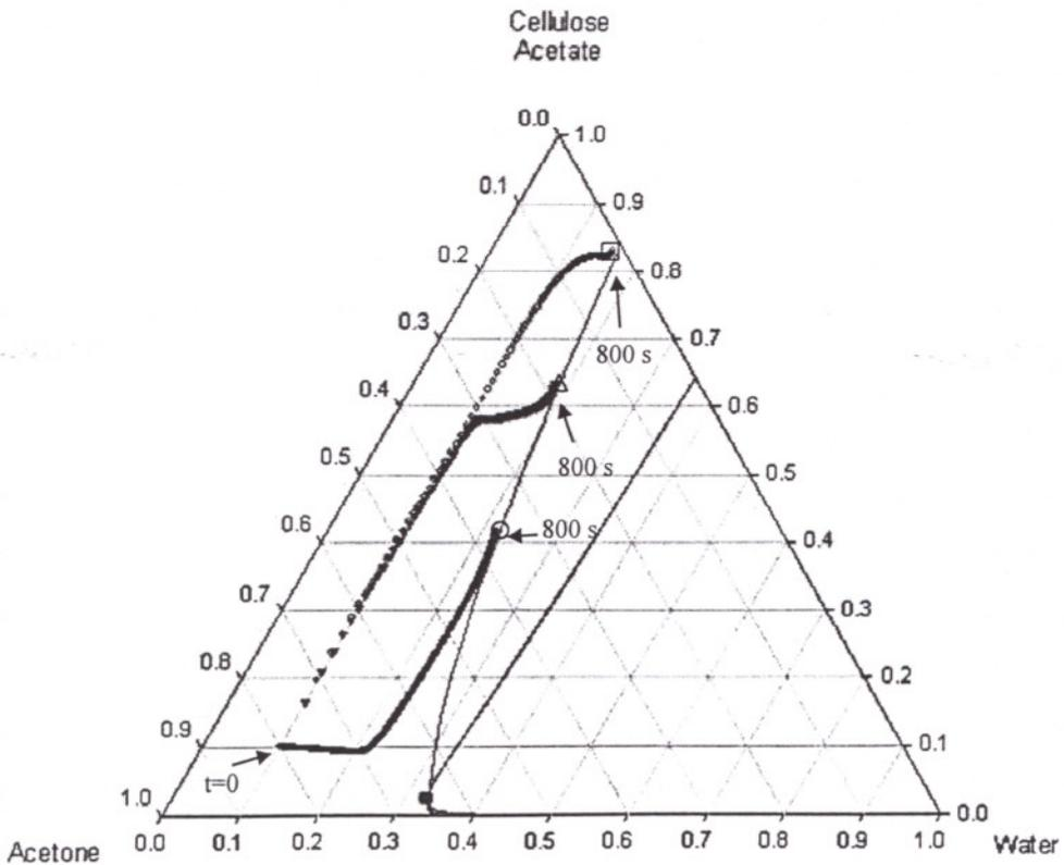
Figure 6.26. Concentration paths of water, acetone and CA for case R8 (O: solution/substrate interface, □: solution/air interface, Δ: point just below solution/air interface).
