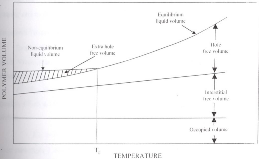
Figure 4.1. Characteristics of the volume of a polymer above and below the glass transition temperature.
