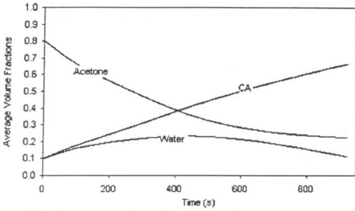
Figure 6.8. Average volume fractions of water, acetone and CA during membrane formation for case R4.
