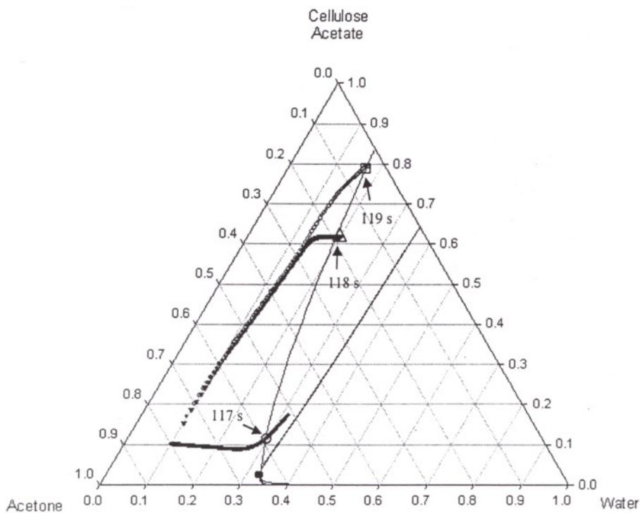
Figure 6.27. Concentration paths of water, acetone and CA for case R9 (O: solution/substrate interface, □: solution/air interface, Δ: point just below solution/air interface).
