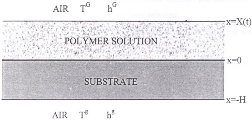
Figure 5.1. Schematic of dry casting process.
