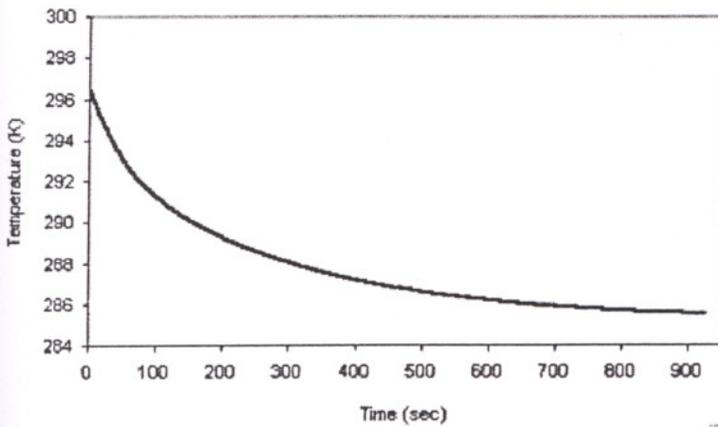
Figure 6.10. Temperature of the solution during membrane formation for case R4.
