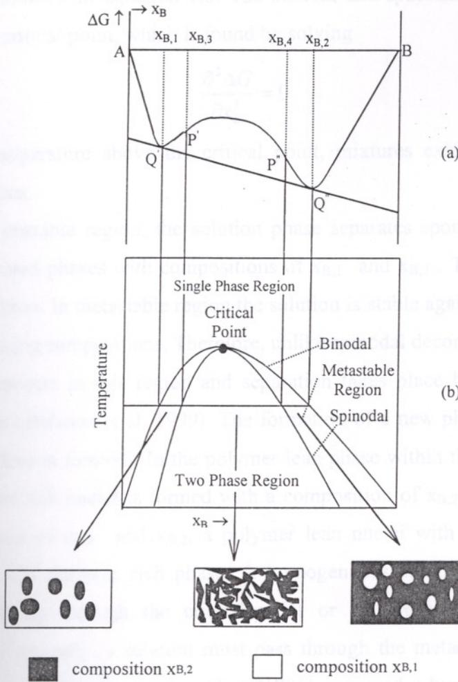
Figure 3.3. (a) Free energy curve and (b) Phase diagram for a binary system and possible structure formation in different parts of the phase diagram.
