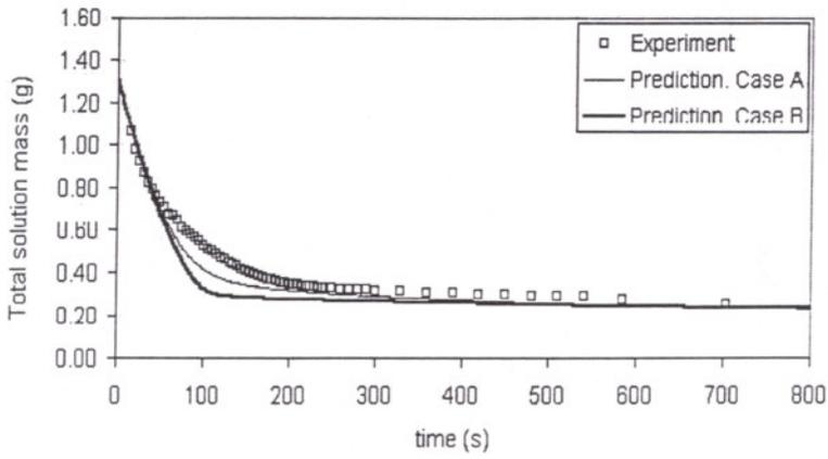
Figure 6.31. Experimental corresponding to case R1, and simulation results for total solution mass as a function of time. The line corresponds to full model, whereas the dashed solid line represents the solution when the cross diffusion coefficients are assumed to be negligible.
