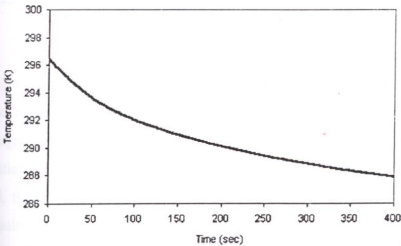
Figure 6.17. Temperature of the solution during membrane formation for case R5.
