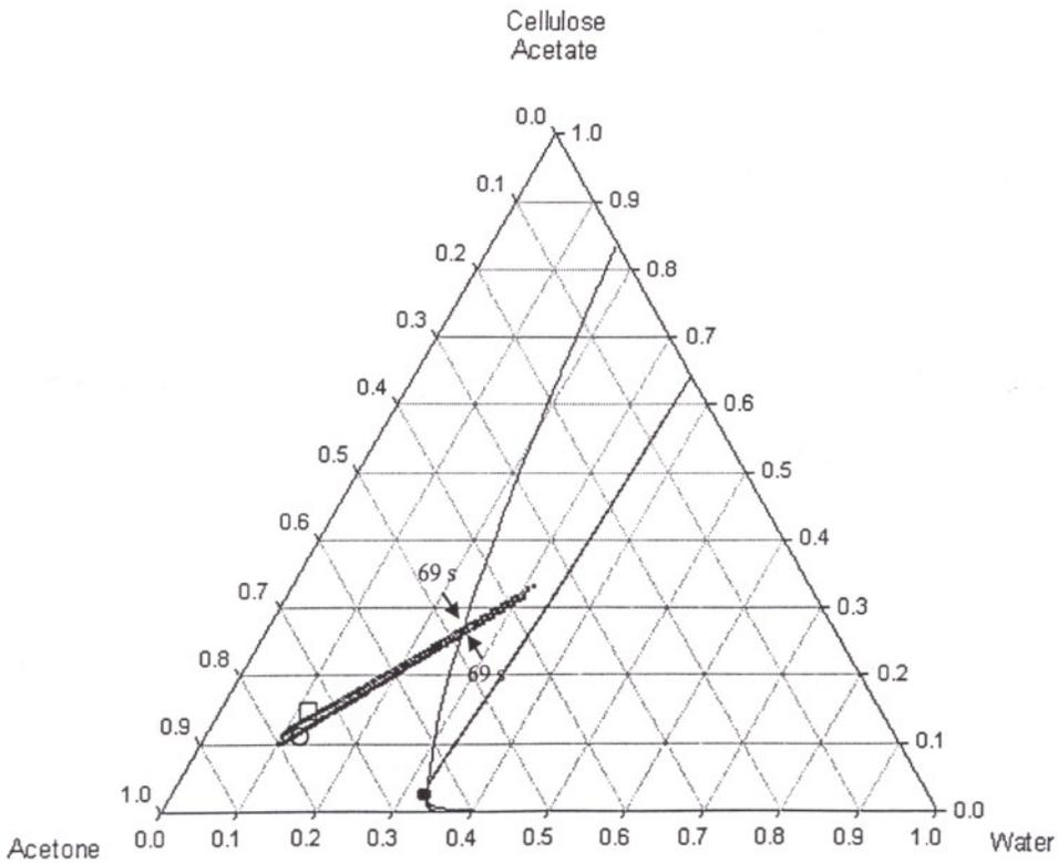
Figure 6.35. Concentration paths of water, acetone and CA for case B (○: solution/substrate interface, □: solution/air interface).
