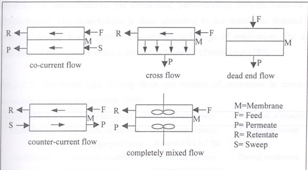
Figure 2.1. Types of ideal continuous flows used in membranes operations.
