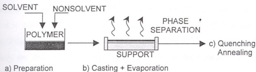
Figure 3.1. Basic steps in phase inversion techniques.
