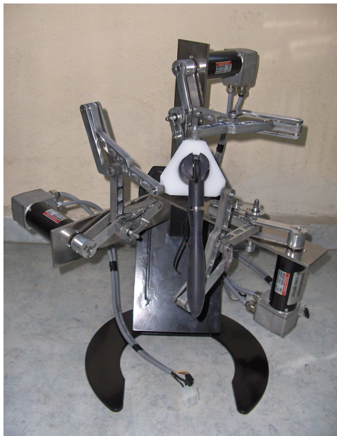
Figure 6.12. Modified 6-DOF mechanism
