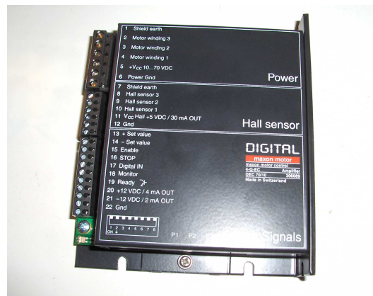
Figure 6.3. Selected maxon motor amplifier
