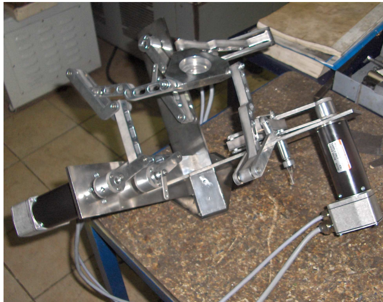
Figure 5.17. Assembled translation mechanism
