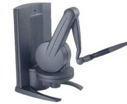
Figure 2.9. PHANTOM® Desktop™ Haptic Device (Source: Sensable 2010)
