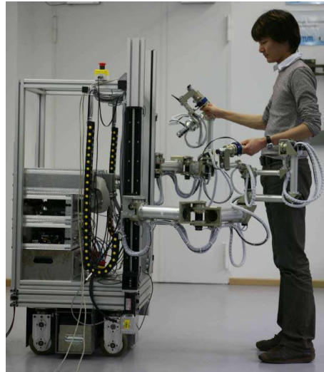
Figure 3.3. Mobile haptic interface VISHARD7 (Source: Peer and Buss 2008)
