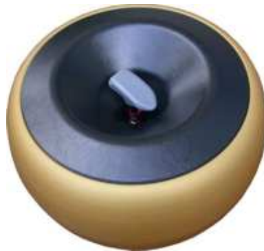
Figure 3.17. Magnetic levitation haptic interface (Source: Butterflyhaptics 2010)
