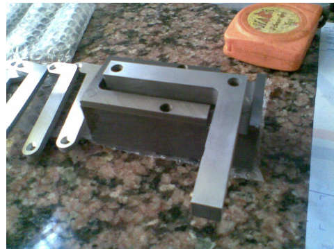
Figure 5.5. Custom gage for bearing houses
