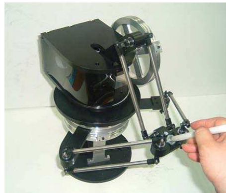
Figure 2.5. Prototype of 3-DOF parallel-type haptic device (Source: Kim, et al. 2007)
