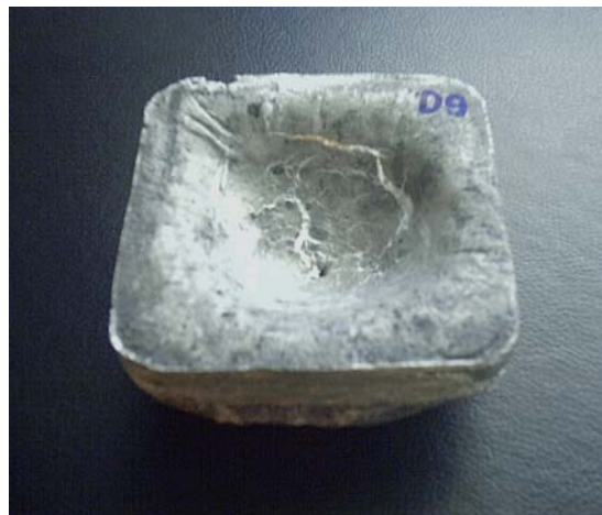
Figure 6.4 A typical geometrical defect in foamed precursor.
