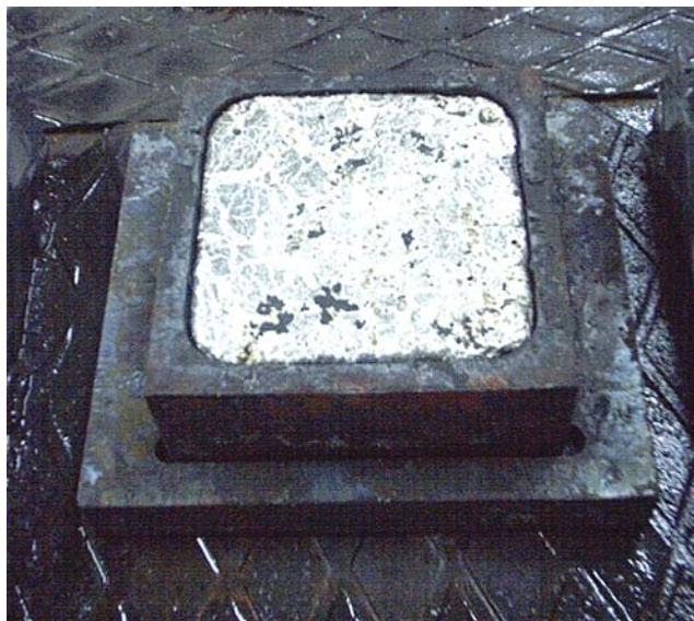
Figure 4.7 Liquid Al foam taken from the furnace after filling the mold.
