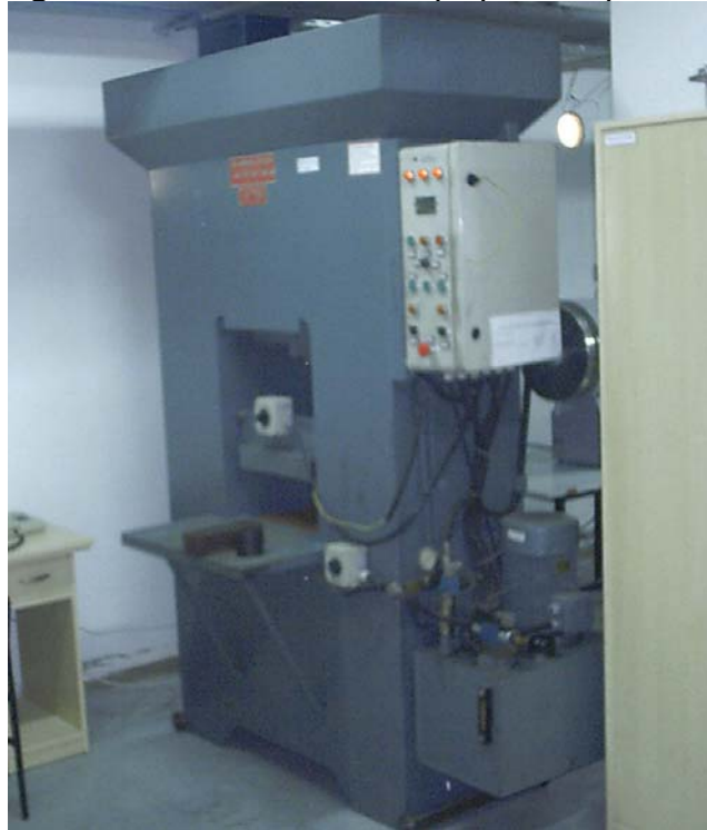
Figure 4.1 Hydraulic press (100 tons) used for compact preparation.
