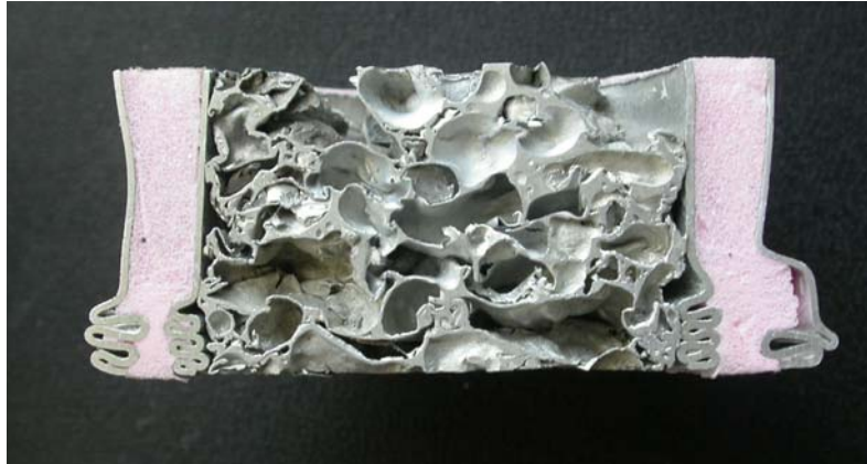
Figure 6.25 Crushed BPA series specimen.
