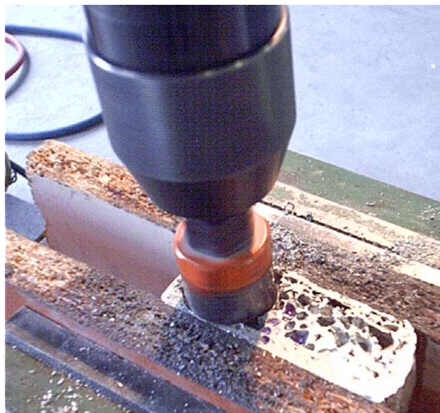
Figure 4.11 Core-drilling normal to foaming direction.
