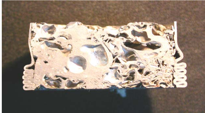
Figure 6.16 Interior view of axisymmetric deformation of Al foam-filled Al tube.
