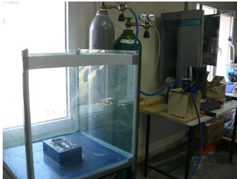
Figure 3.2. Oxygen concentration measurement system used in this study.
