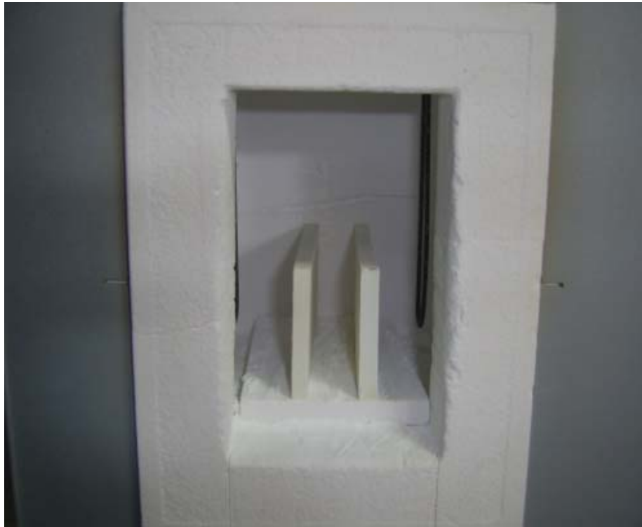
Figure 3.5. Placement of the large plate samples in the oven
