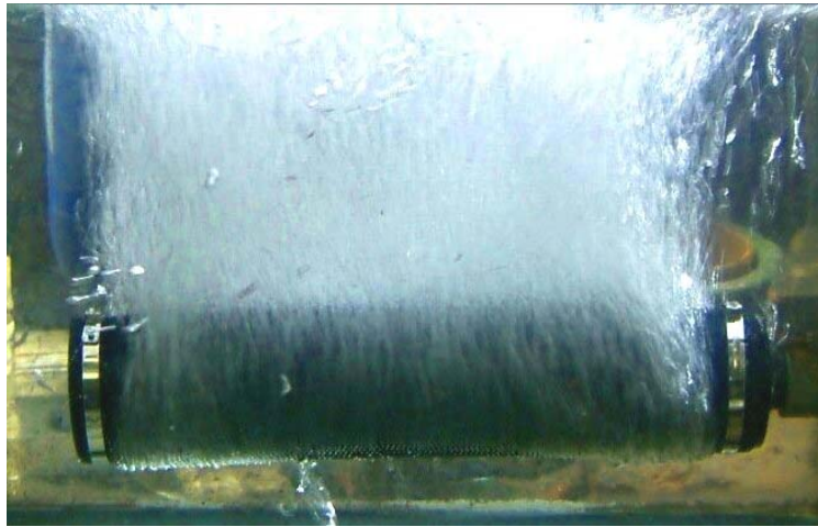
Figure 2.2. Photograph of air diffuser (Source: Dryden Aqua 2009)
