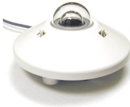
Figure 5.12 Kipp & Zonen Pyranometer used in IZTECH solar radiation measurements [36].
