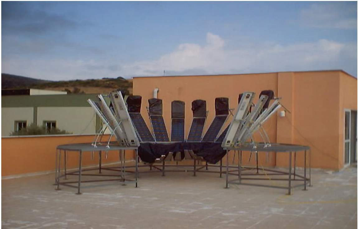
Figure 6.24 Omega Type Solar Charge Station Experiments without Reflectors.
