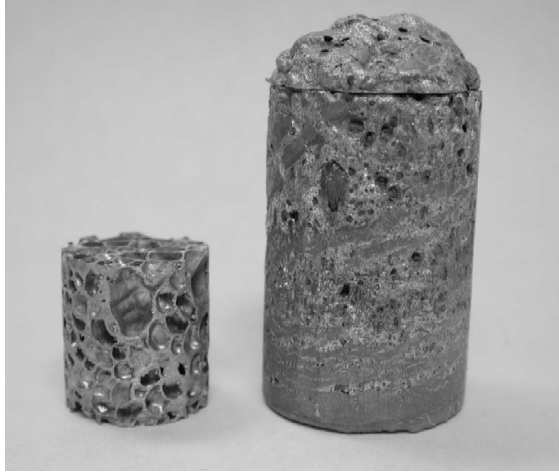
Figure 4.2 Cylindrical compression test sample (left) and the original foam specimen from which the test sample was core-drilled (right).
