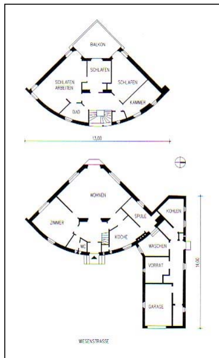
Figure 2.34. The plans of the Taut House by Bruno Taut, Berlin, 1926-1927 (Source: Brenne, Tomisch, Borgert & Celasun 2005: p. 111)
