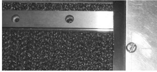
Figure 2.11. Rail and Block
