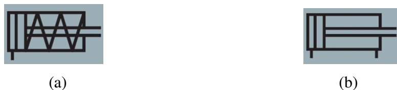
Figure 2.2. Basic cylinder types and symbols (a) Single Acting Cylinder (b) Symbol Double Acting Cylinder
