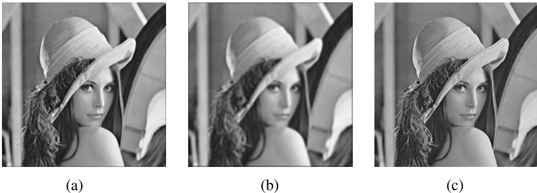
Figure 3.2. Smoothing nonnoisy image (a) Lena.gif (b) Filtered with sigma = 1 (c) Filtered with sigma = 3
