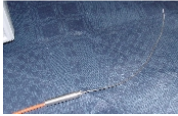
Figure 4.4. Pt-Rh-Pt, S-type thermocouple probe
