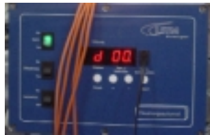
Figure 4.2. DUNGS electronic unit with microprocessor for controlling the burner operation
