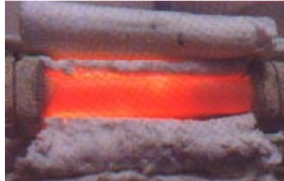
Figure 3.8. Radiant burner with pure oxygen on porous burner basis [22]
