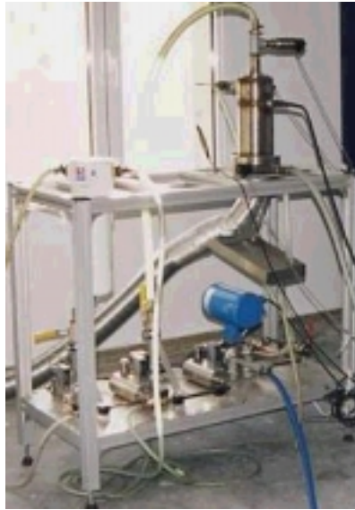
Figure 4.19. 10 kW Porous Medium Combustor test rig
