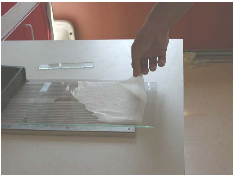
Figure 5.5. Separation of PLA or PDLA Composite Films from the Glass Surface.
