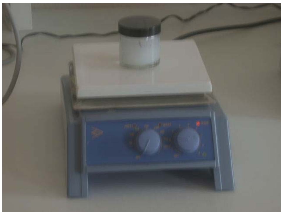
Figure 5.2. Mixture of PLA or PDLA –HA Composites on Magnetic Stirrer at T_{\text{room}} .
