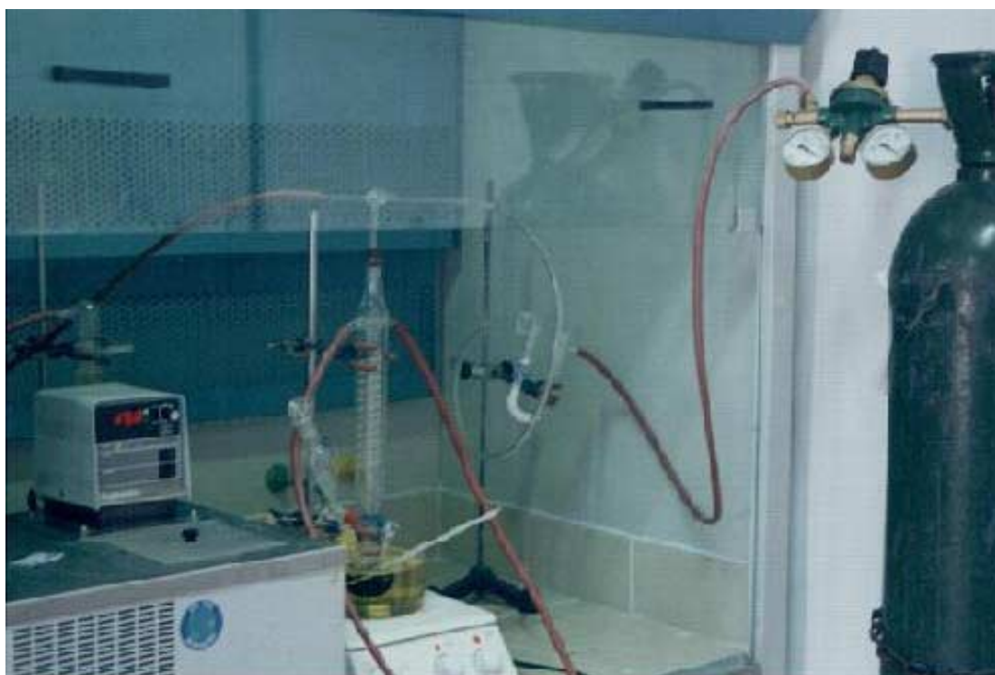
Figure 4.2. Experimental set-up designed for acylation of 2-MN reactions
