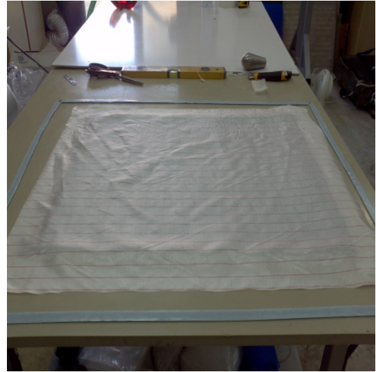
Figure 3.1. Laying out of fabrics on the infusion table and application of peel-ply material
