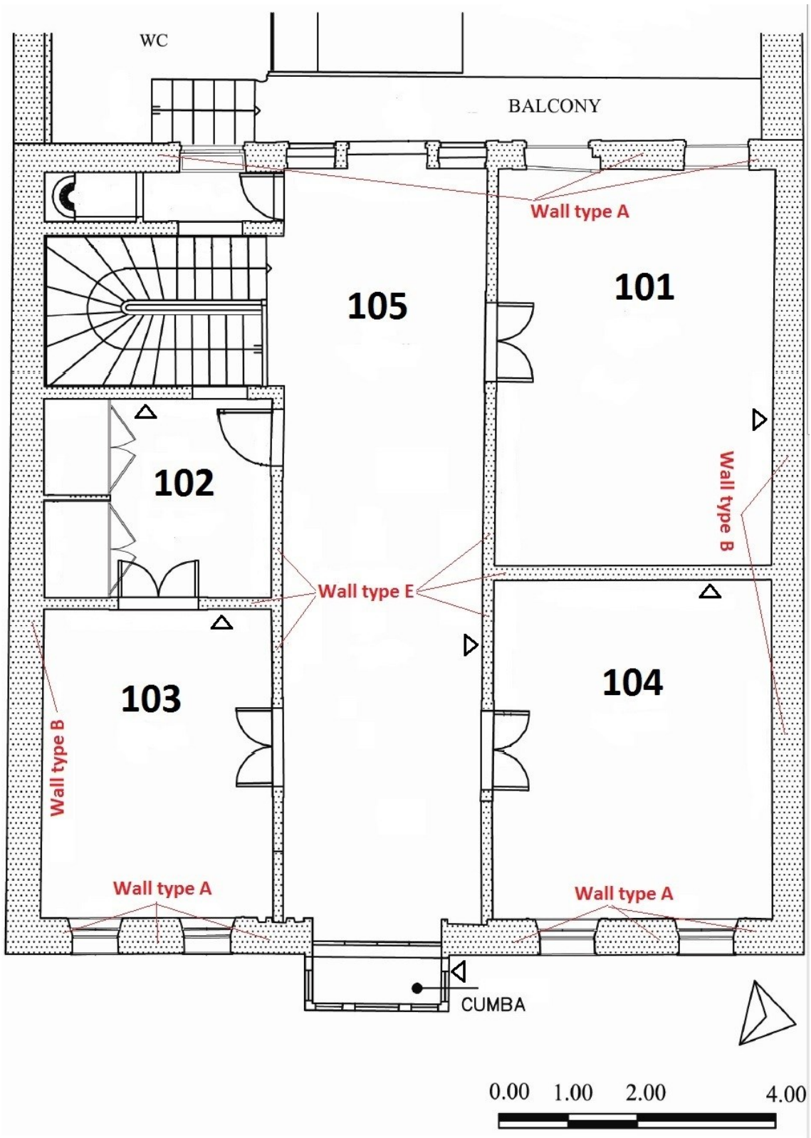
Figure 3.5. First floor plan (Modified from the drawings provided by Dept. of Architectural Restoration - IZTECH)
