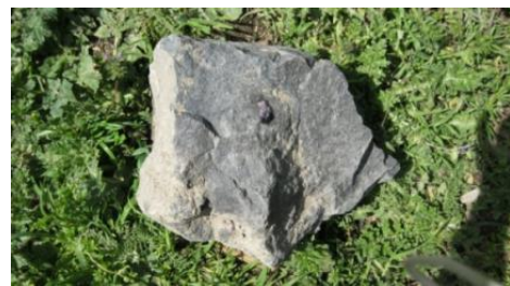
Figure 121. The karataş used on foundation
