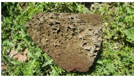
Figure 120. The köfeke stone used as a filling material
