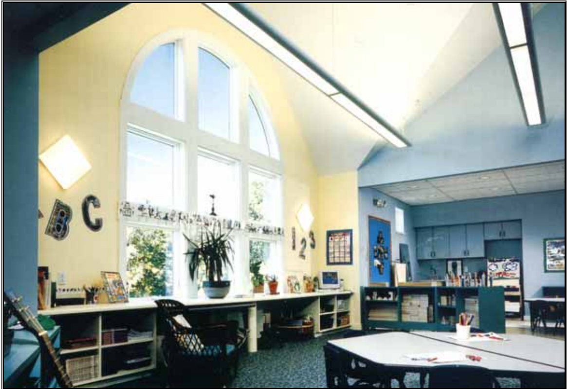
Fig.3.9. Photograph shows natural light use in a classroom. Fluorescent lamps are also hanging from the ceiling for equal lighting. Rumsey Hall School, Washington Depot, Connecticut.
