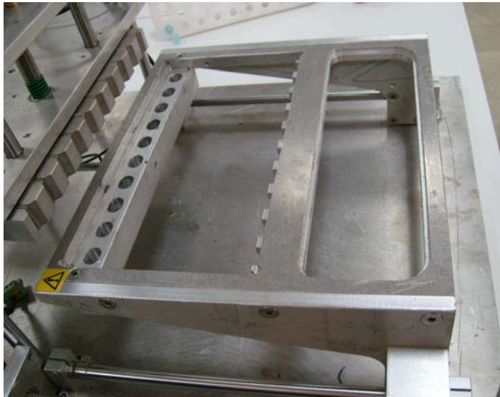
Figure C.2. The work table and the heater block.
