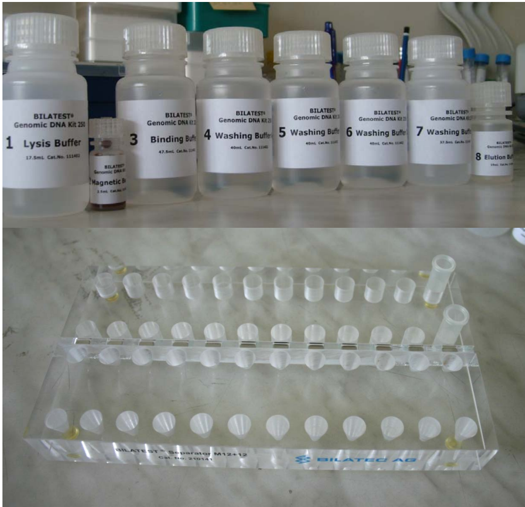
Figure 3.12. View of BILATEST® Genomic DNA Kit 250 for extraction of DNA with 8 chemicals and magnetic separator
