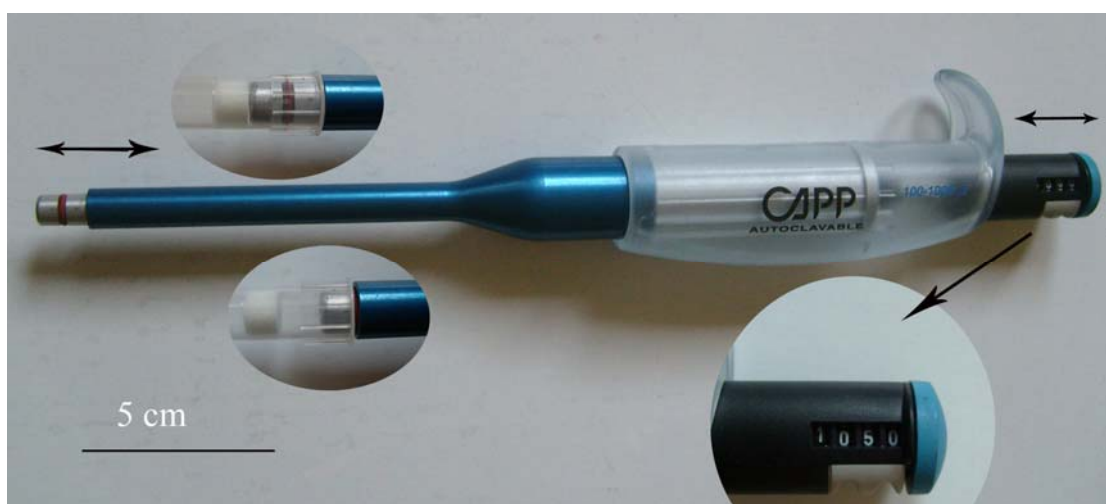
Figure 3.6. Picture of 100-1000 \mu\text{l} pipette and mechanisms of application.
