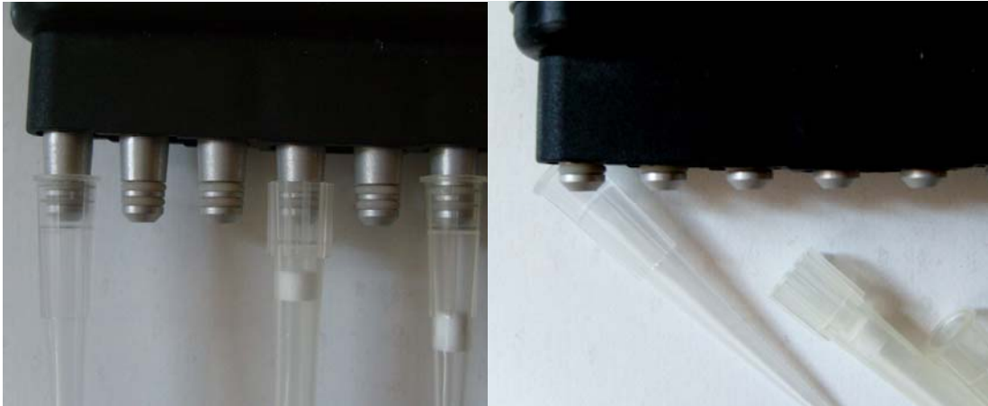
Figure 3.9. 20-200 \mu l Multy head hand pipetter and pipette tip extracting mechanism.
