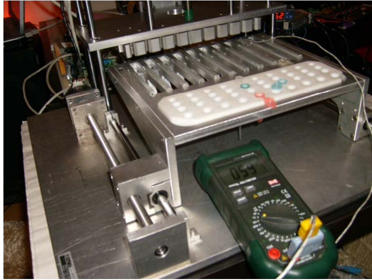
Figure 6.2. Temperature test of the heating unit
