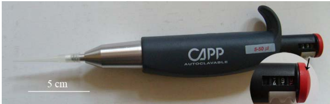
Figure 3.7. Picture of 5-50 µl pipetter with 50 µl pipette and volumetric scale.
