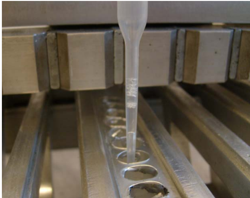
Figure 6.4. Bubbles in the pipette tip.
