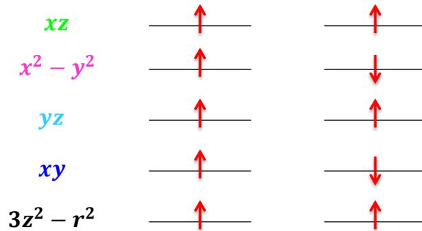
Figure 4.2. High spin state and low spin state of Co  $3d^5$ .
